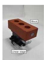
(a) Block and linear stage that generates precise behavior
