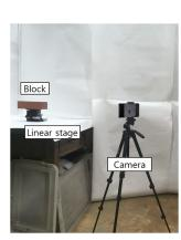
(b) Experimental setup of camera
