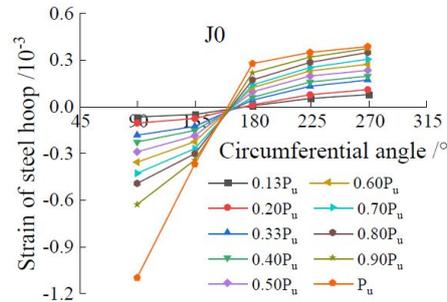
Fig. 4 Strain distribution of steel hoop in J0
