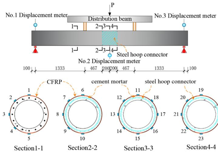
(b) Schematic diagram of measuring points in reinforced specimens (mm)
