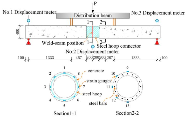
(a) Schematic diagram of measuring point in J0 (mm)
