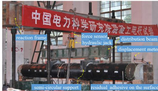
Fig. 1 Photo of test setup
