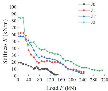
Fig. 8 Stiffness degeneration curves
