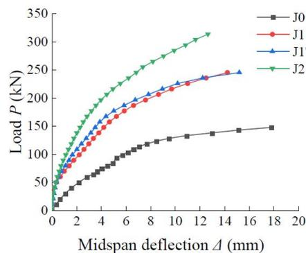
Fig. 6 Load-midspan deflection curves
