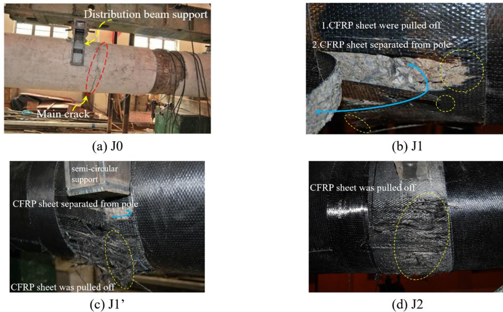
Fig. 3 Failure mode of each specimen with connector
