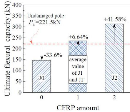
Fig. 7 Comparison of ultimate bearing capacity
