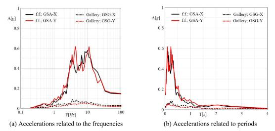
Fig. 4 Response spectra in terms of accelerations of the measurements recorded during the L'Aquila 2009 Earthquake in the stations GSA (external to the mountain) and GSG (inside the Gallery).f.f.: free field, Gallery: inside the Gallery. X and Y are both horizontal directions orthogonal to each other
