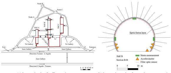
(a) Layout in plan for fiber optic sensors
