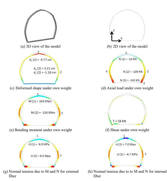
Fig. 3 Numerical modeling of the transversal cross section
