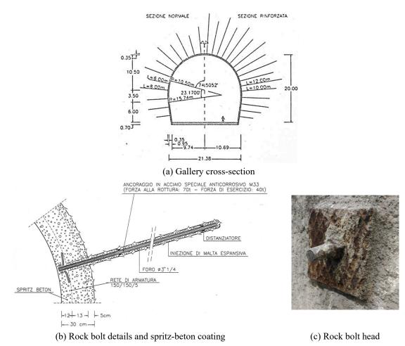
Fig. 2 Consolidation interventions in the galleries designed by Lunardi (1990) and actual condition of a rock bolt head in a picture taken in an accessible point of galleries
