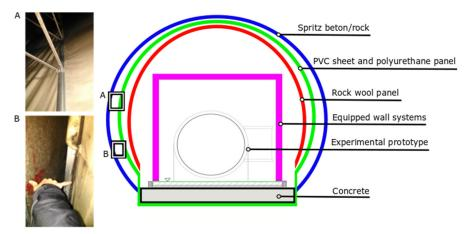
Fig. 5 Sketch of gallery cross section evidencing the interspace between spritz beton/rock layer and polyvinyl chloride (PVC) panels: detail A shows the aluminum structure, detail B the interspace length (≅ 20 cm)
