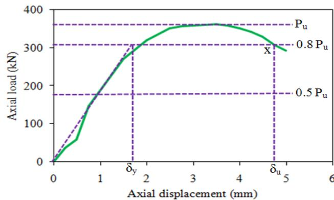
Fig. 10 Procedures for ductility calculation
