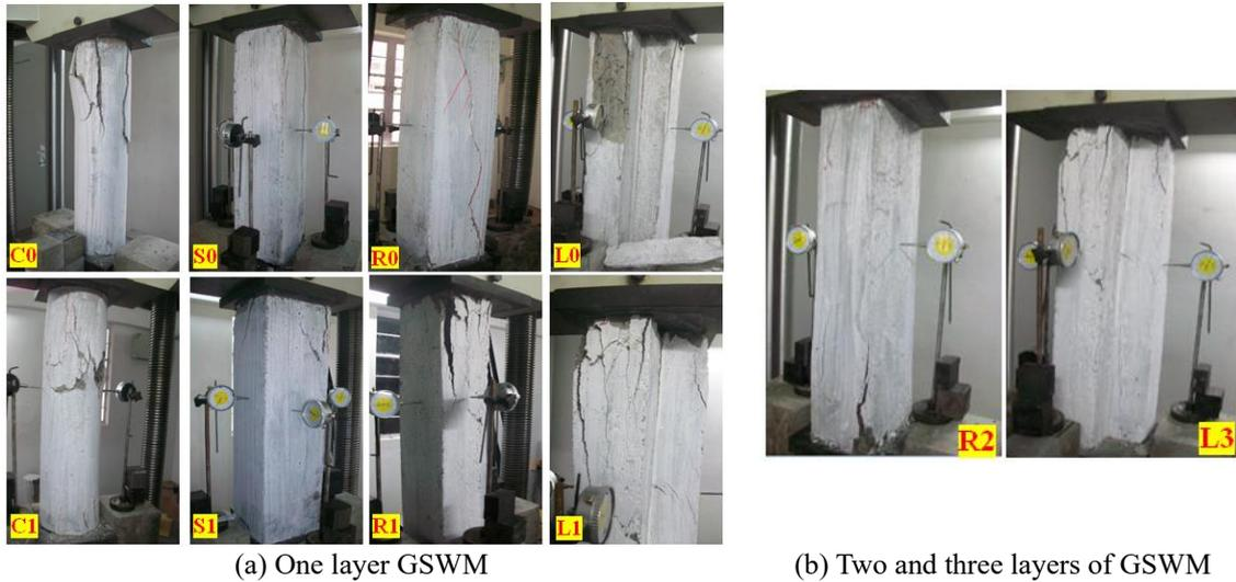
Fig. 6 Failure of tested specimens
