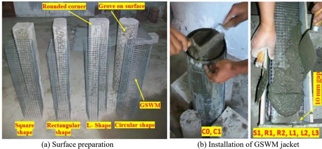
Fig. 4 Casting of specimens
