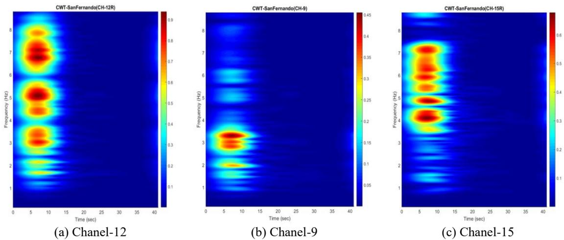
Fig. 10 Spectrogram of data recorded from San Fernando earthquake at Ch-12, Ch-9 and Ch-15 in radial direction along the foundation of the dam
