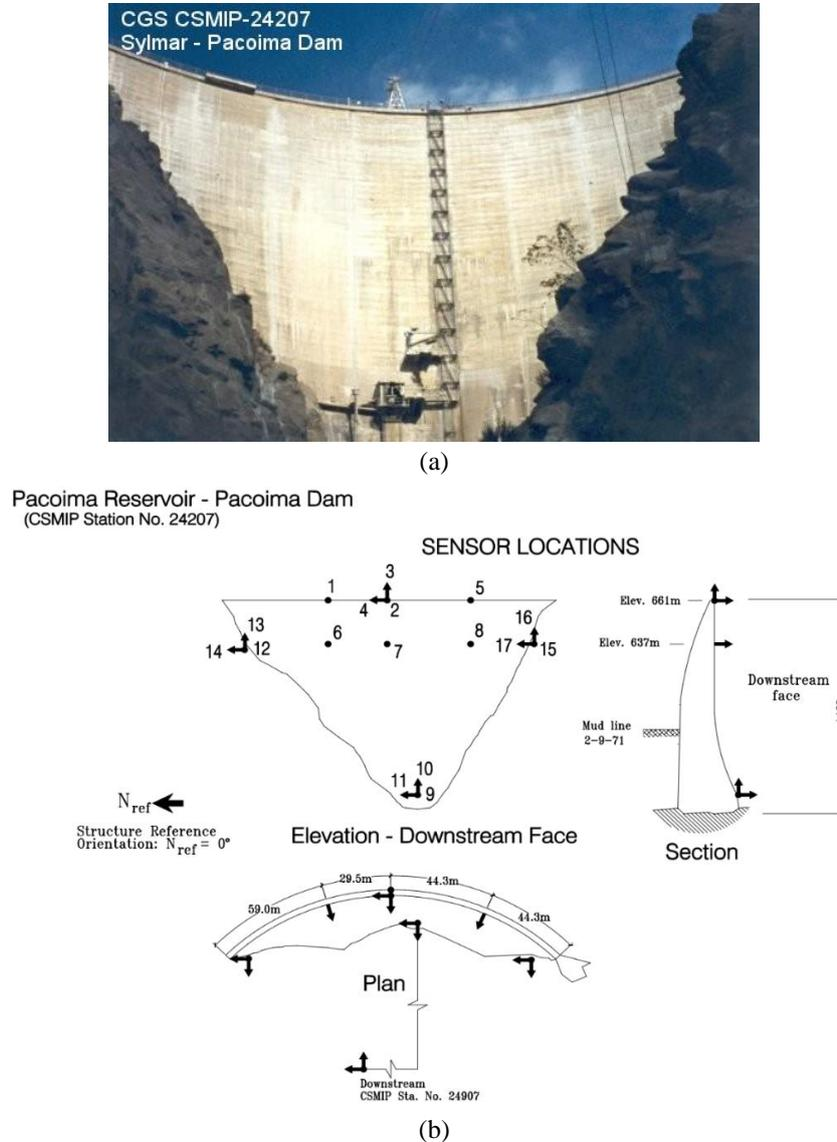
Fig. 1 (a) Photo of the Pacoima dam and (b) Distribution of seismometers on the Pacoima dam
