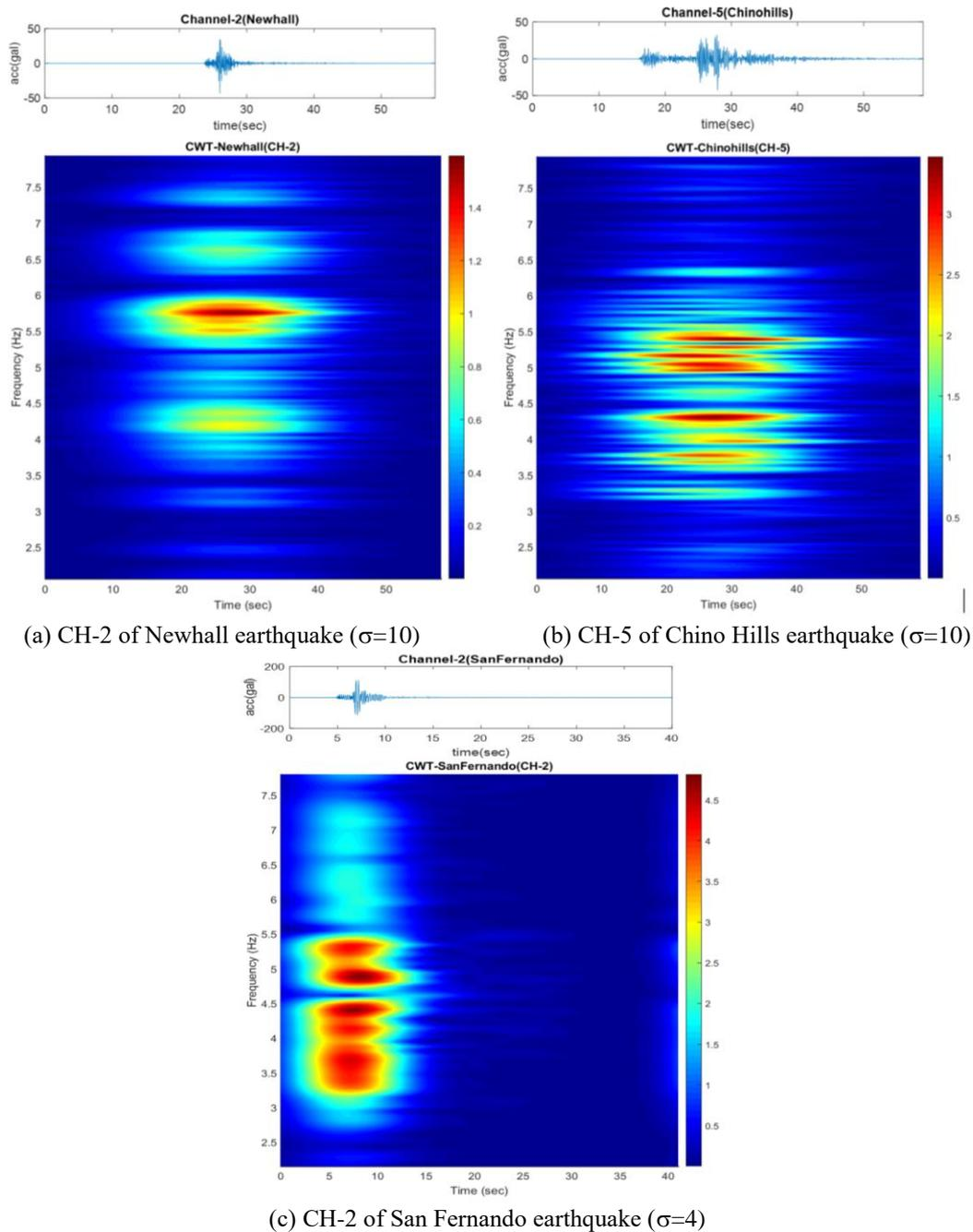
Fig. 8 Spectrogram of three seismic event data recorded from Pacoima dam
