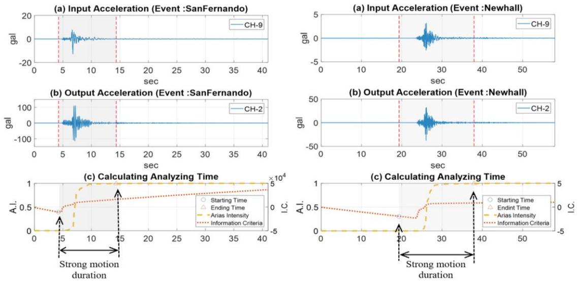
Fig. 4 Example to determine the strong motion duration for subspace identification; (a) & (b): Shaded area indicated the selected strong motion duration for analysis, (c) using IC index and 99.5% of Arias Intensity to determine strong motion duration
