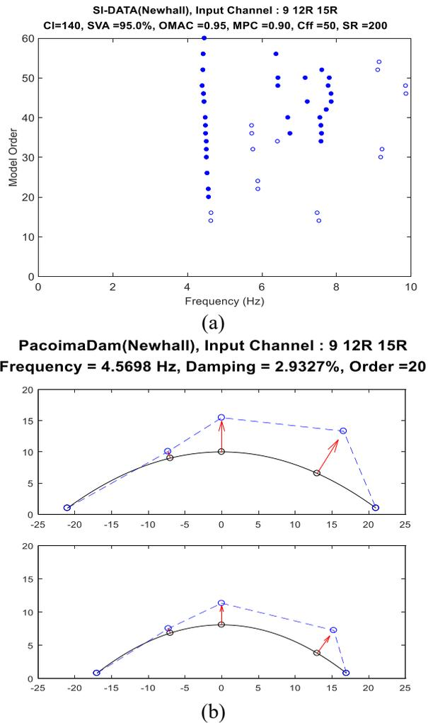
Fig. 7(a) Stability diagram from using Newhall earthquake data (using cl=140) and (b) Identified mode of the Pacoima dam from Newhall earthquake data (at level 661 m and 637 m)
