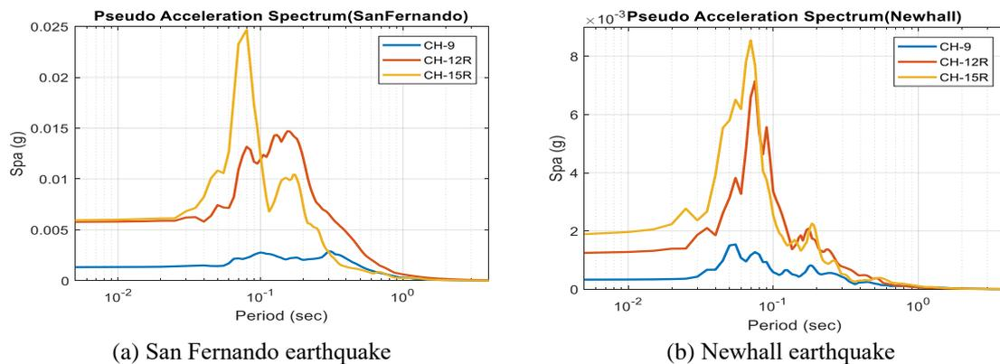
Fig. 3 Acceleration response spectrum of two set of seismic data from the dam abutment
