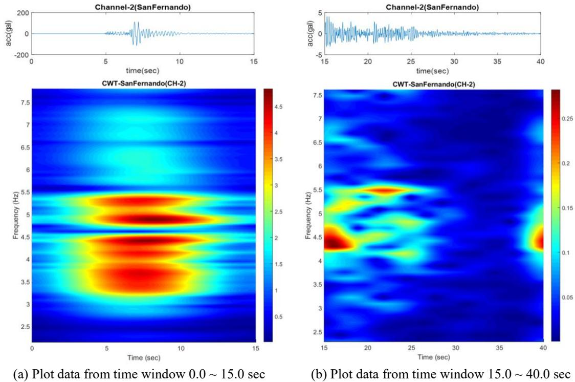
Fig. 9 Spectrogram of Chanel 2 data of Pacoima dam recorded from San Fernando earthquake
