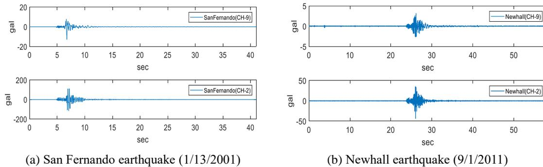
Fig. 2 Recorded acceleration at Channel 2 and Channel 9 of Pacoima dam
