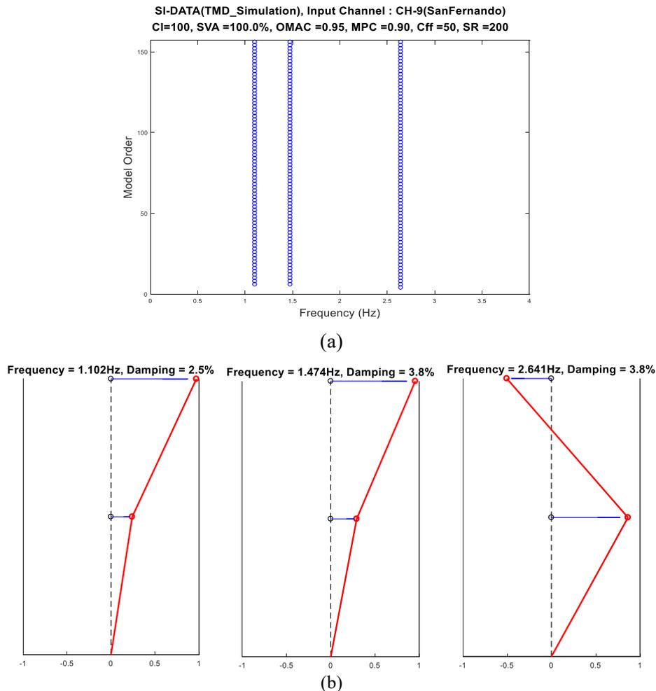
Fig. 12 (a) Stabilization diagram using response data from the 3-DOF system (with tuned mass) and (b) Identified mode shapes from the simulated TMD system.
