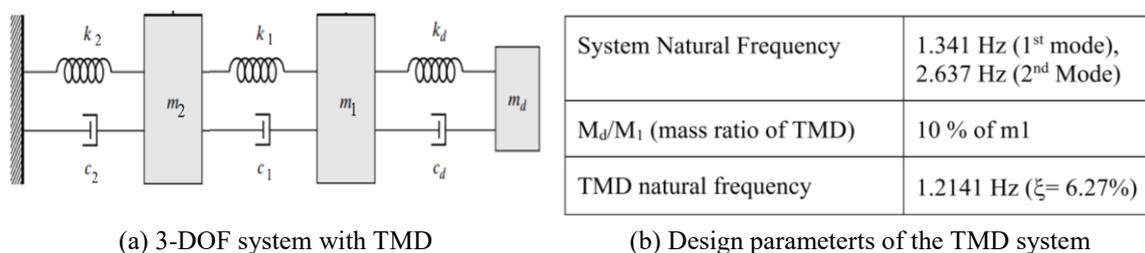
Fig. 11 Simulation of 2-DOF system with tuned mass
