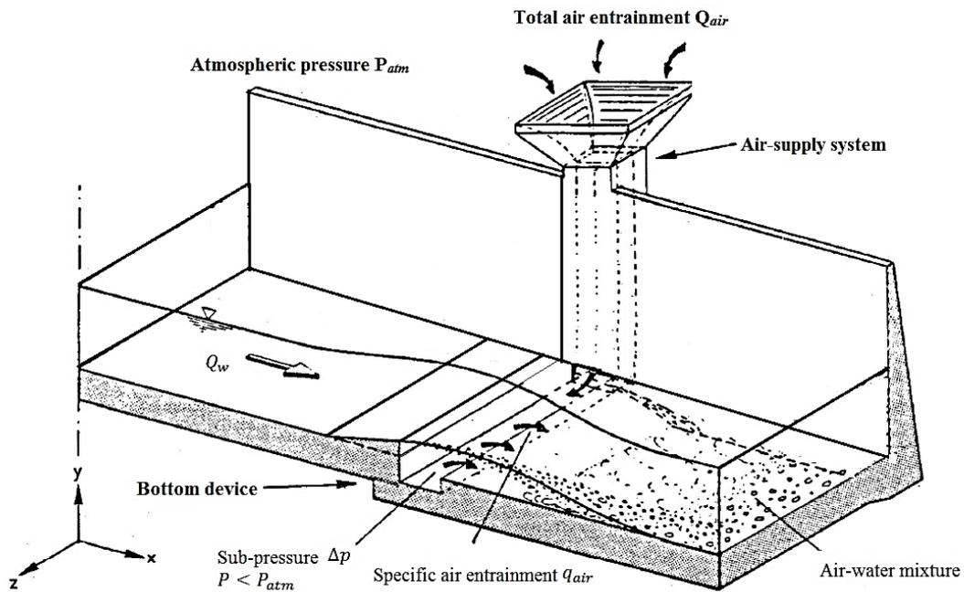
Fig. 8 A typical spillway aerator (Volkart and Rutschmann 2018)
