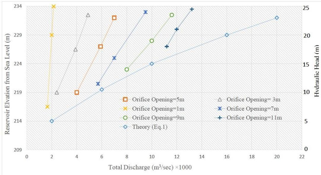
Fig. 6 Karkheh dam's spillway total discharge capacity
