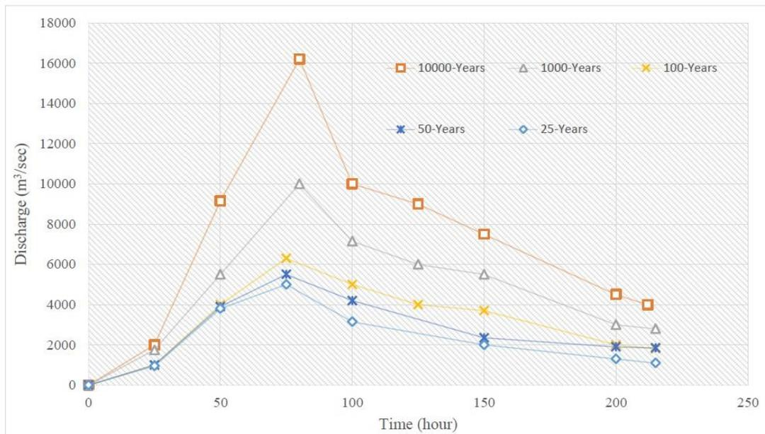
Fig. 7 Karkheh Dam's flood hydrograph
