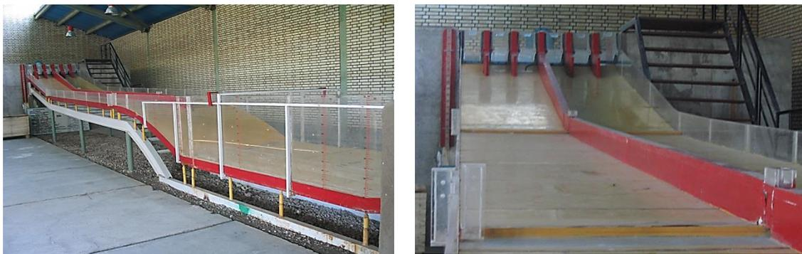
Fig. 10 1/64 scale model of Karkheh Dam's spillway
