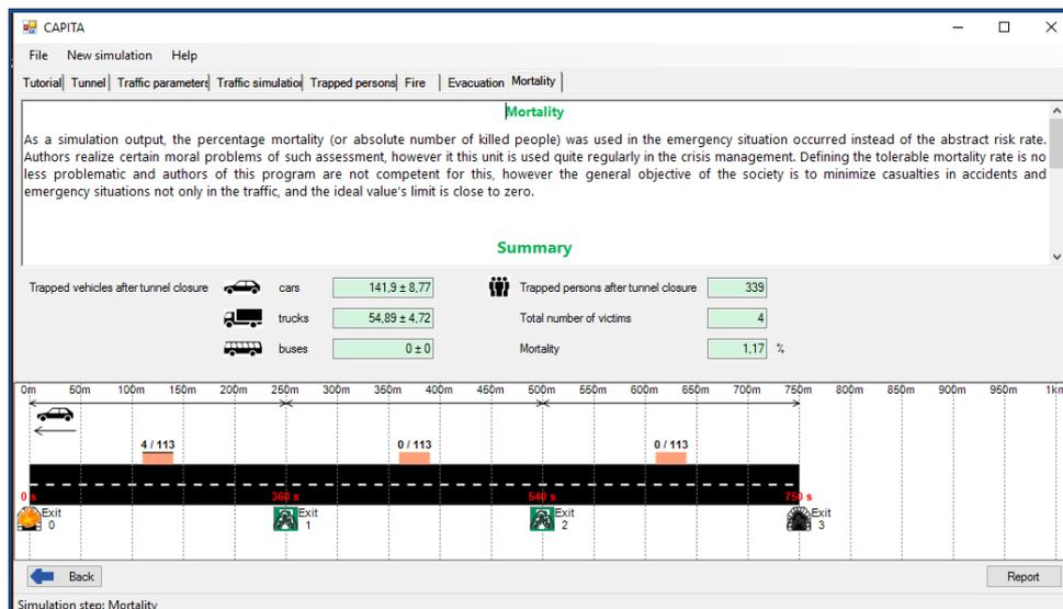
Fig. 6 CAPITA 1.5 user interface - final workflow step with tunnel visualization and mortality calculation (critical times on particular exits in red, victims shown as black columns)
