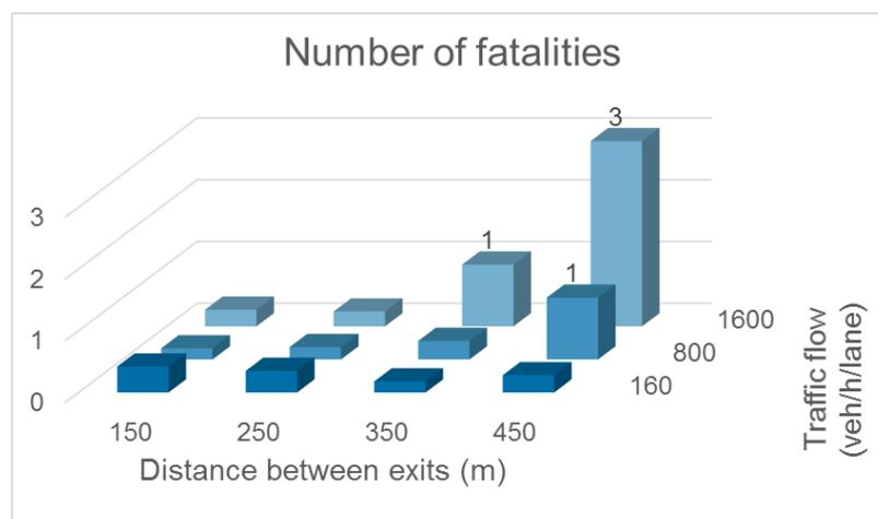
Fig. 2 An example showing the number of fatalities as related to distance between exits and traffic density
