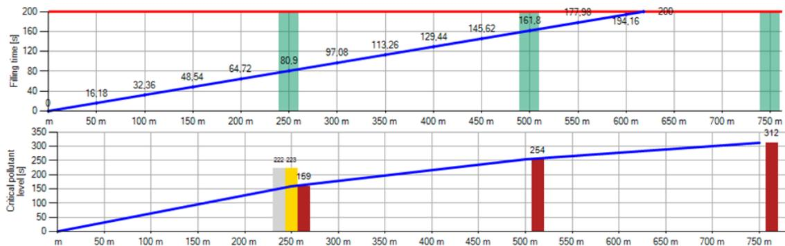
Fig. 4 (above) The tunnel filling time as result of traffic microsimulation model. Exits located every 250 m are highlighted in green. The time to the tunnel closure (200 s) is depicted as a red line); (below) Critical times [s] for CO propagation in grey and HCL propagation in yellow according to smoke propagation model and the custom physical model in brown
