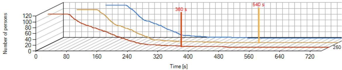
Fig. 5 The number of people leaving the tunnel in time (evacuation process) for different distances between exits (red - 250 m, yellow - 500 m and blue - 750 m). Vertical lines depicts the critical time when the particular exit is blocked due to critical pollutant concentration
