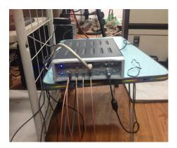
Fig. 6 Data acquisition instrument of LMS Test.Lab
