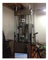
(a) The material servo instrument MTS810
