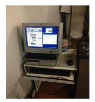
(b) The control terminal TestStar IIs
