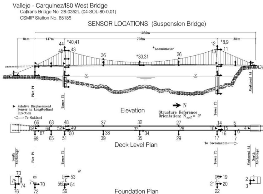
Fig. 8 Alfred Zampa bridge instrumentation (<http://www.strongmotioncenter.org>)
