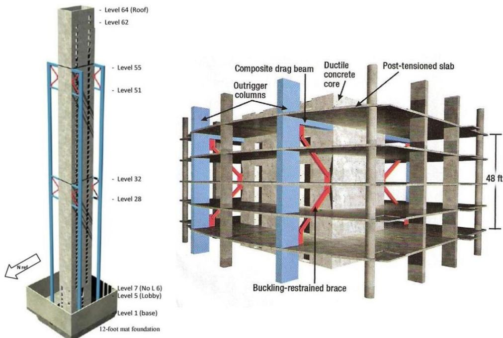
Fig. 3 One Rincon Hill Tower structural system (Huang *et al.* 2012)
