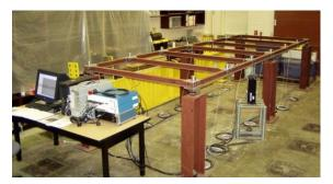
Fig. 1 Experimental setup of the UCF Benchmark Structure (adopted from Gul and Catbas 2008)
