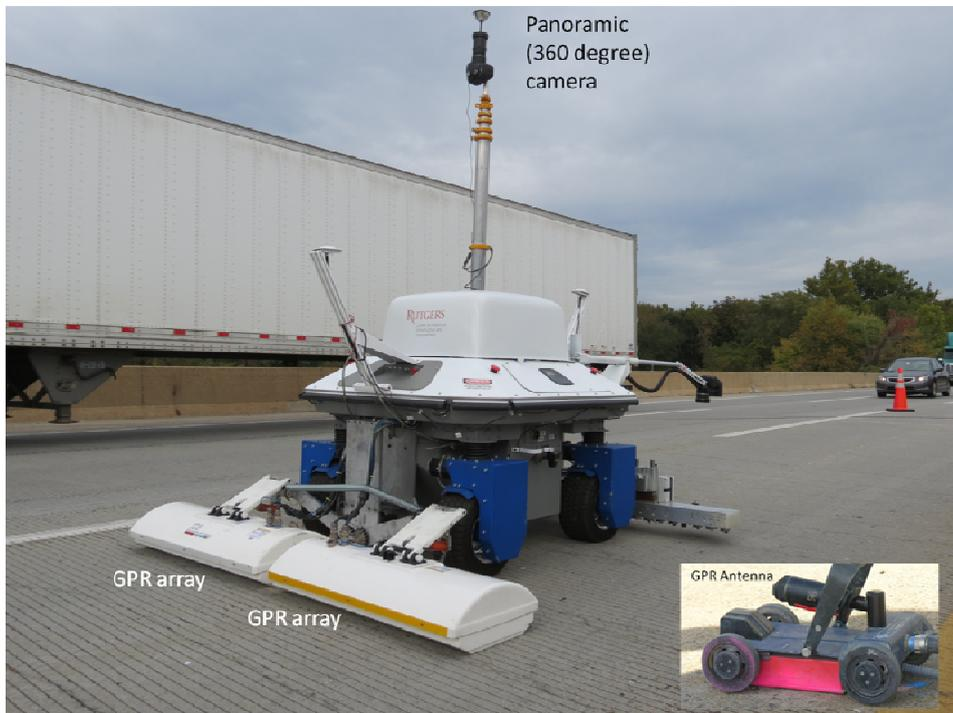
Fig. 3 Back side of RABIT with two GPR arrays and mast with a panoramic camera
