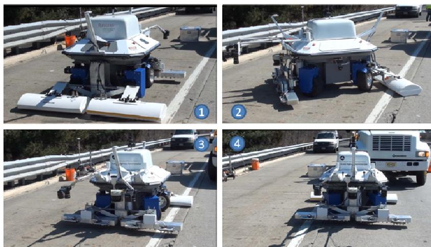
Fig. 4 Sample path planning and RABIT movement during surveys
