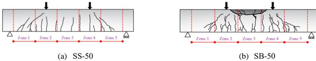
Fig. 5 Schematic of crack propagation at failure: (a) SS-50 and (b) SB-50
