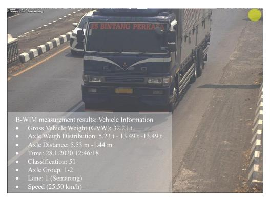
Fig. 5 Vehicle information from B-WIM measurements (Pawiro Baru A Bridge, Site ID001)
