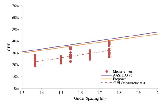
Fig. 7 Relationships between GDF and girders spacing, single lane loading
