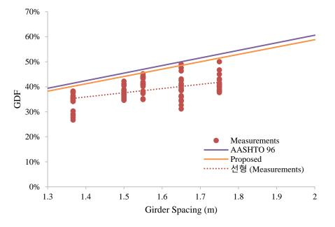
Fig. 8 Relationships between GDF and girders spacing, two-lane loading
