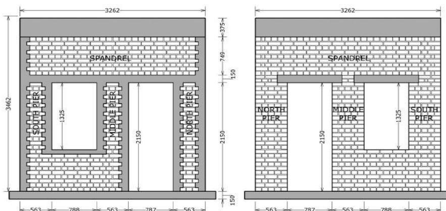
Fig. 7 Confined masonry walls and Unreinforced masonry walls (source: Ashraf *et al.* 2012)
