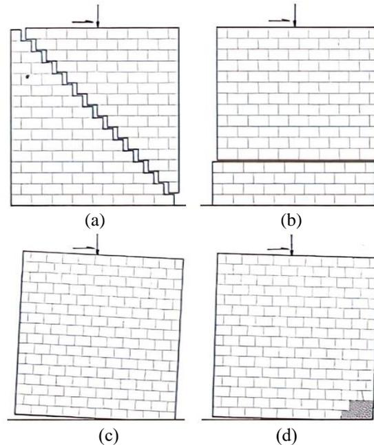
Fig. 5 In-plane failure modes of a laterally loaded URM wall: (a) shear failure, (b) sliding failure, (c) rocking failure and (d) toe crushing. (ElGawady *et al.* 2006)
