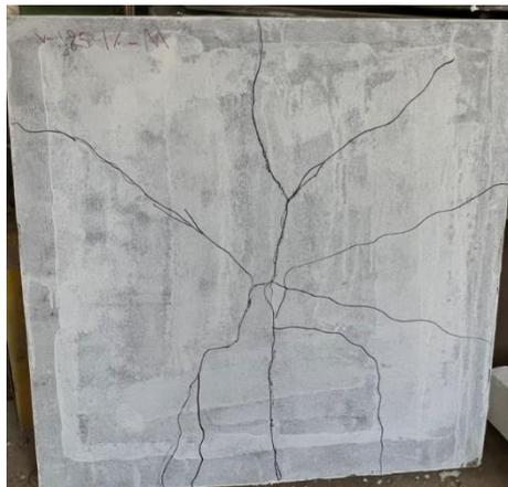
Fig. 28 Failure pattern of (V-125-1%-M)
