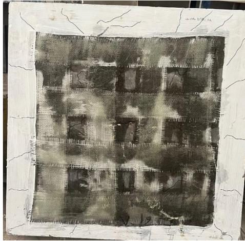
Fig. 27 Failure pattern of (V-125-2GF-M)
