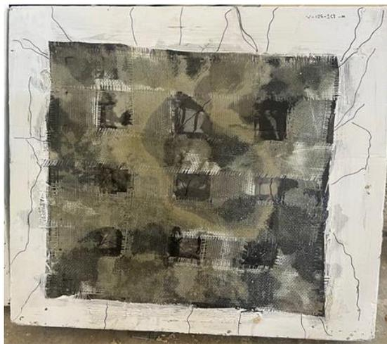
Fig. 26 Failure pattern of (V-125-1GF-M)
