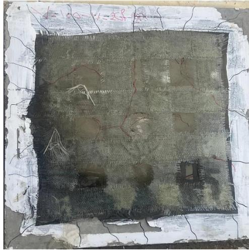
Fig. 30 Failure pattern of (V-100-2GF-1%-M)
