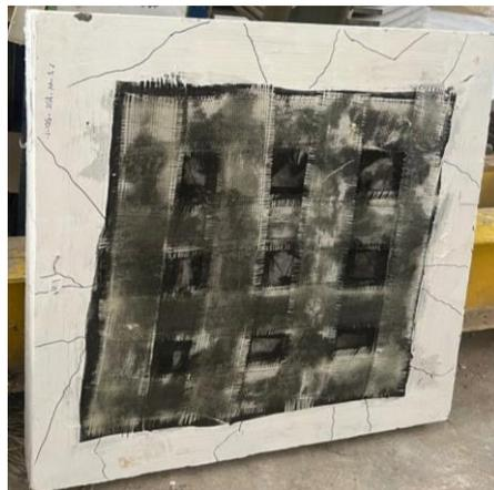
Fig. 29 Failure pattern of (V-125-2GF-1%-M)
