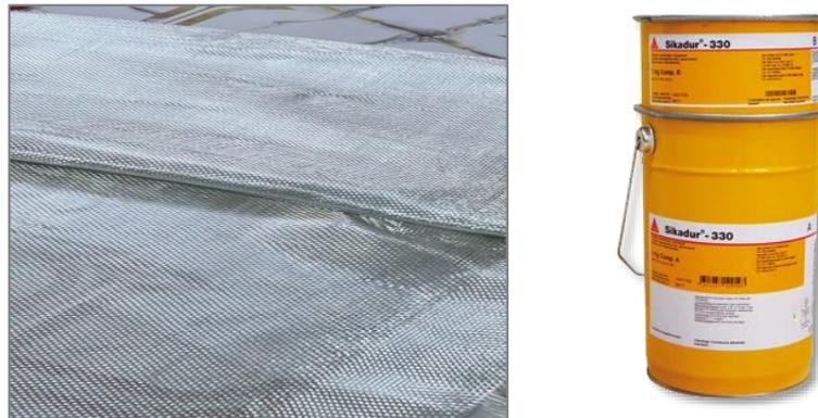
Fig. 3 Sample of GFRP sheet and Epoxy resin Sikadur-330
