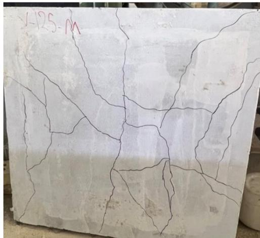
Fig. 24 Failure pattern of (V-125-M)
