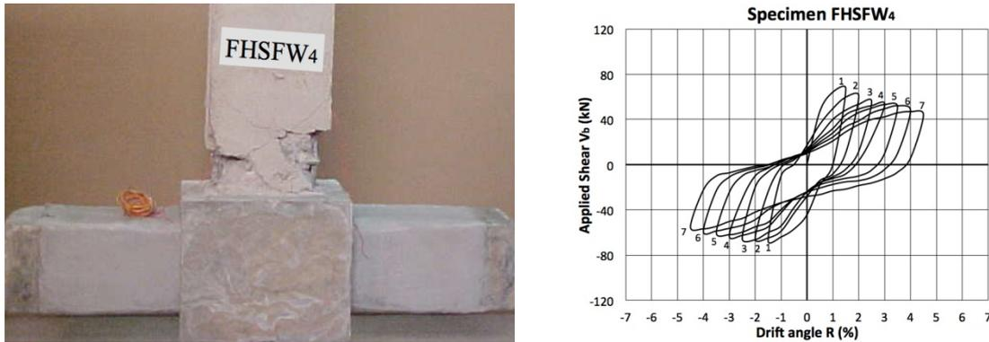
Fig. 7 Plots of applied shear versus drift angle and failure mode of the strengthened subassembly FHSFW<sub>4</sub>
