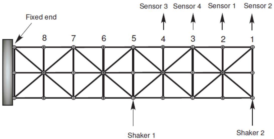
Fig. 9 Plan view of the schematic of the four meters long NASA eight bay truss structure
