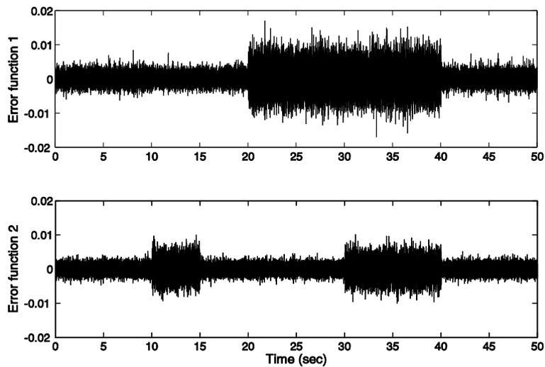
Fig. 7 Actuator error function from sensors 2 and 3's measurement using direct method 1 with  $p=40$ : (a) actuator 1, and (b) actuator 2
