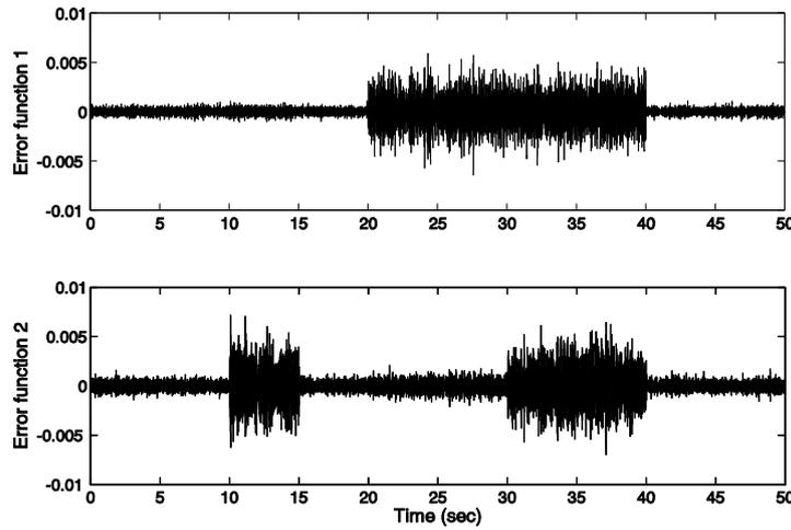
Fig. 4 Actuator error function from sensors 2 and 4's using direct method2 with  $p=40$ : (a) actuator 1, and (b) actuator 2
