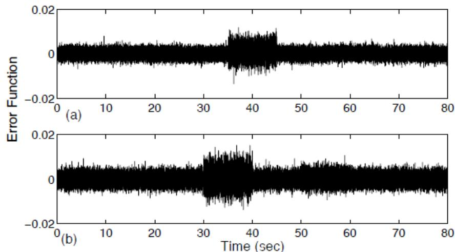
Fig. 10 Sensor error function for uncertain sensors 1 and 2 using direct method 1 with  $p=40$ : (a) uncertain sensor 1, and (b) uncertain sensor 2
