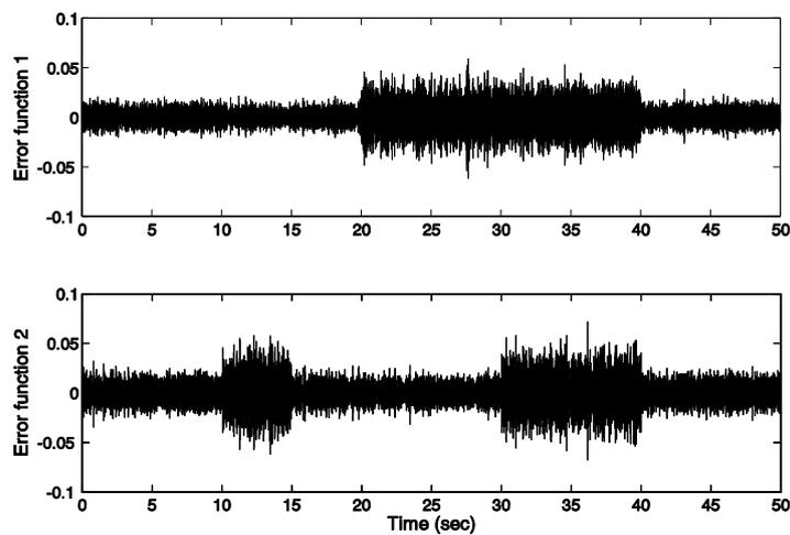
Fig. 2 Actuator error function from sensors 2 and 4's measurements using indirect method with  $p=40$ : (a) actuator 1, and (b) actuator 2
