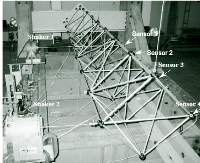
Fig. 1 Picture of an Eight Bay Truss Structure
