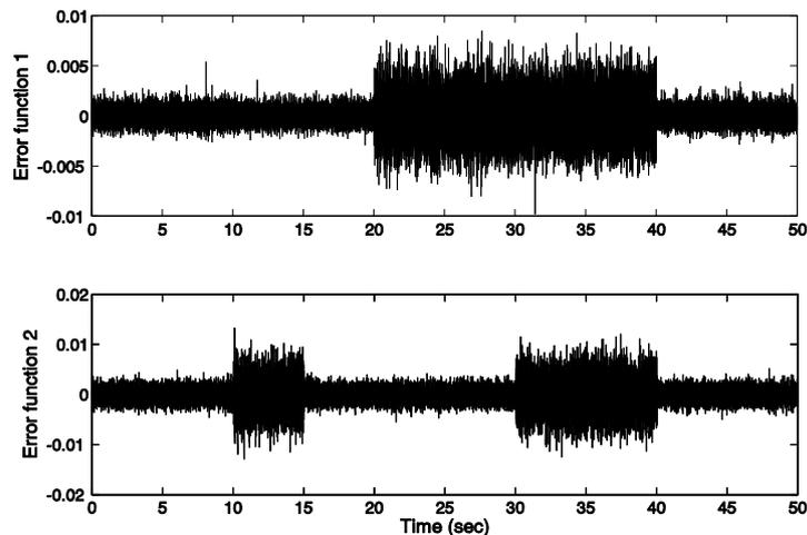
Fig. 3 Actuator error function from sensors 2 and 4's measurement using direct method 1 with  $p=40$ : (a) actuator 1, and (b) actuator 2
