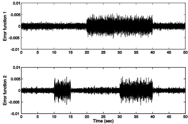
Fig. 8 Actuator error function from sensors 2 and 3's measurement using direct method 2 with  $p=40$ : (a) actuator 1, and (b) actuator 2
