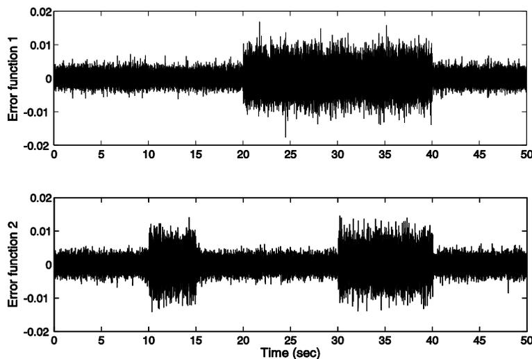
Fig. 5 Actuator error function from sensors 1 and 4's measurement using direct method 1 with  $p=40$ : (a) actuator 1, and (b) actuator 2
