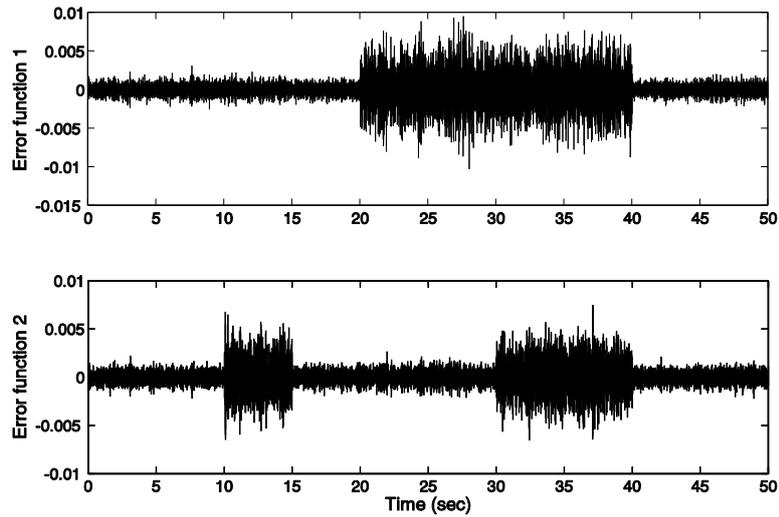
Fig. 6 Actuator error function from sensors 1 and 4's measurement using direct method 2 with  $p=40$ : (a) actuator 1, and (b) actuator 2
