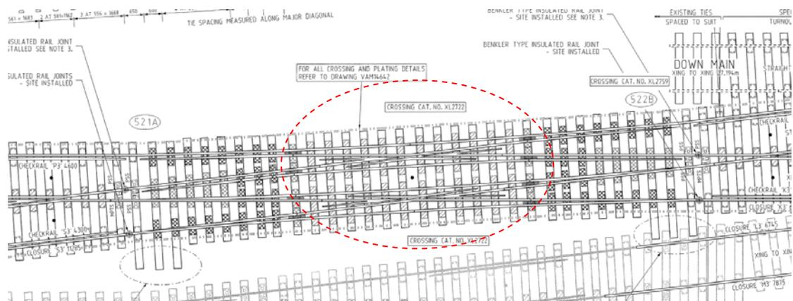
Fig. 4 Field layout of double slips (521/522) at Hornsby NSW
