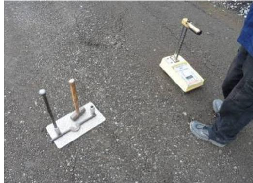
Fig. 8 Compaction test of capping layer
