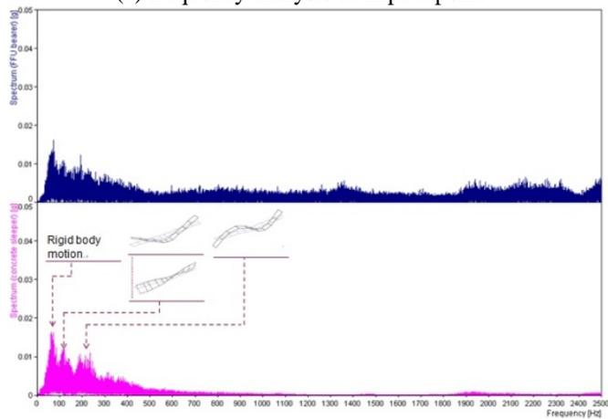
Fig. 14 Vibration data of a pass-by train (Passenger train, X-Up Main)
