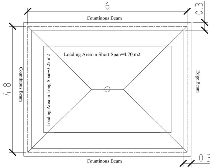
Fig. 3 Block load distribution for half portion in long and short direction of slab orientation
