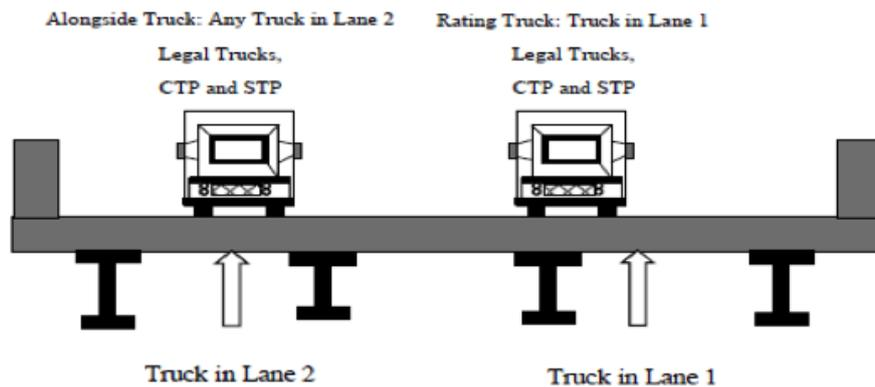
Fig. 11 Maximum loading event calibration for live load factors (Case 2).
