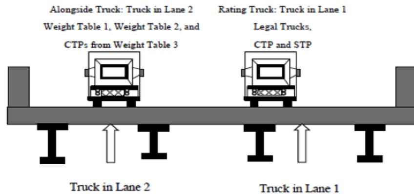
Fig. 10 Maximum loading event calibration for live load factors (Case 1).
