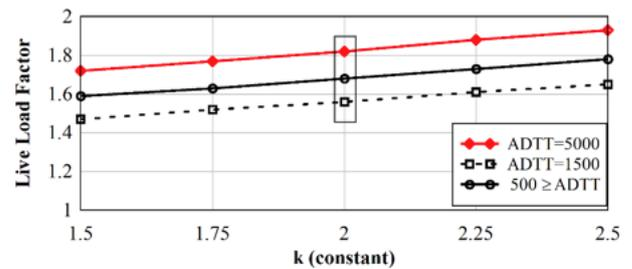
Fig. 9 Largest live load factors found for HS20 loading considering a 5 years of evaluation period
