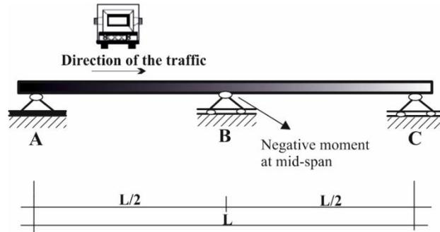
Fig. 3 Negative moment location for 2-span continuous bridge analysis
