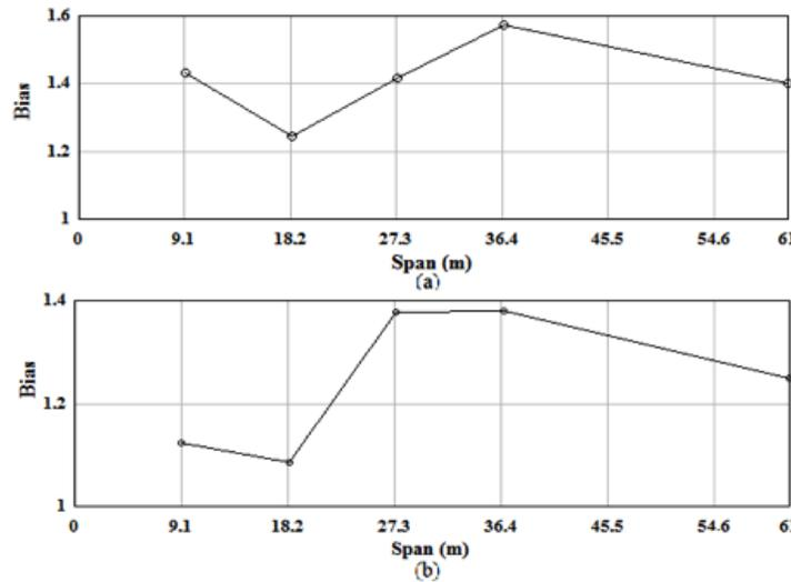
Fig. 8 Live load bias factors for two lane shear per girder (ADTT=5,000).
