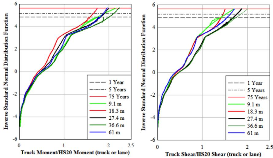
Fig. 4 Moments and shears for simple spans, all year WIM data for I-5 Woodburn NB.
