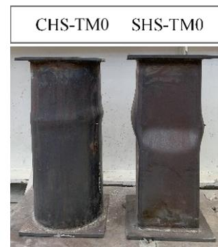
Fig. 12 Hollow columns after the tests
