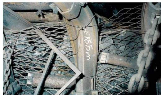
Fig. 1 Deformed mining support (Janas 2008)
