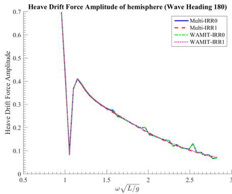
Fig. 17 HEAVE DRIFT FORCE VS  $\omega\sqrt{L/G}$
