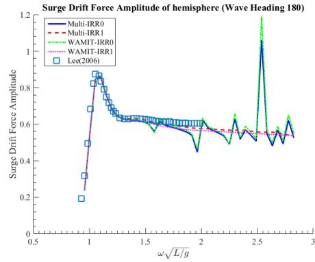
Fig. 16 SURGE DRIFT FORCE VS  $\omega\sqrt{L/G}$
