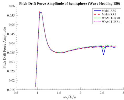
Fig. 18 PITCH DRIFT FORCE VS  $\omega\sqrt{L/G}$
