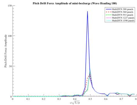
Fig. 10 PITCH DRIFT FORCE VS  $\omega\sqrt{L/G}$
