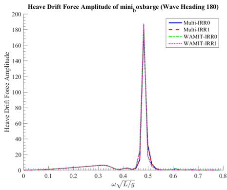
Fig. 13 HEAVE DRIFT FORCE VS  $\omega\sqrt{L/G}$
