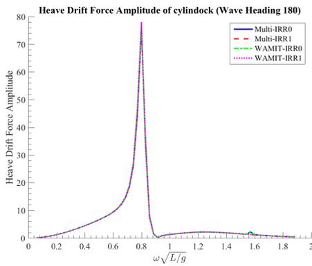
Fig. 21 HEAVE DRIFT FORCE VS  $\omega\sqrt{L/G}$
