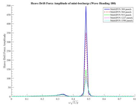
Fig. 9 HEAVE DRIFT FORCE VS  $\omega\sqrt{L/G}$
