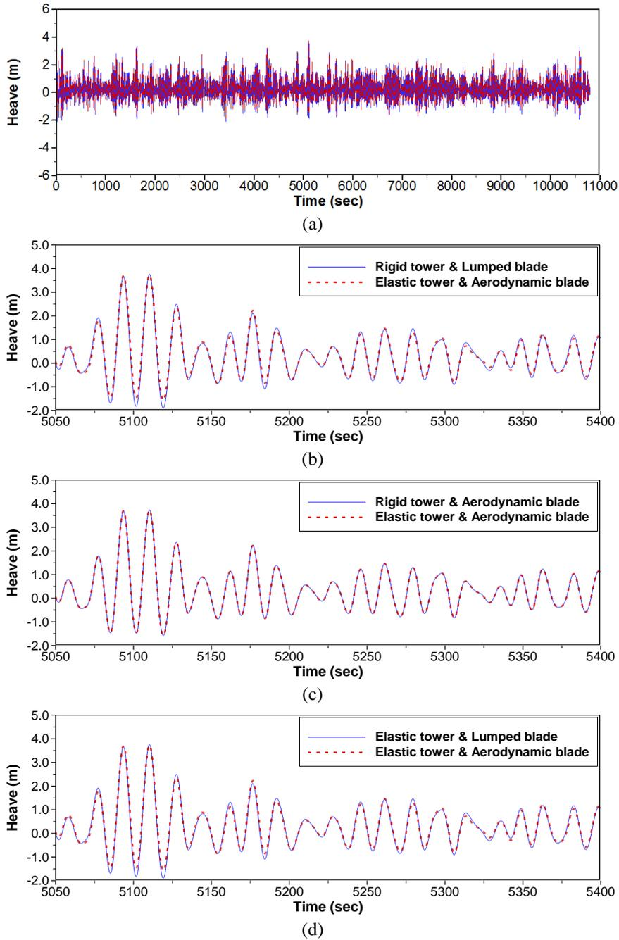
Fig. 9 (a) Comparison of heave in sea state 8 (full range), (b) Comparison of heave in sea state 8 (zoom range : case 1 vs 4), (c) Comparison of heave in sea state 8 (zoom range : case 2 vs 4) and (d) Comparison of heave in sea state 8 (zoom range : case 3 vs 4)
