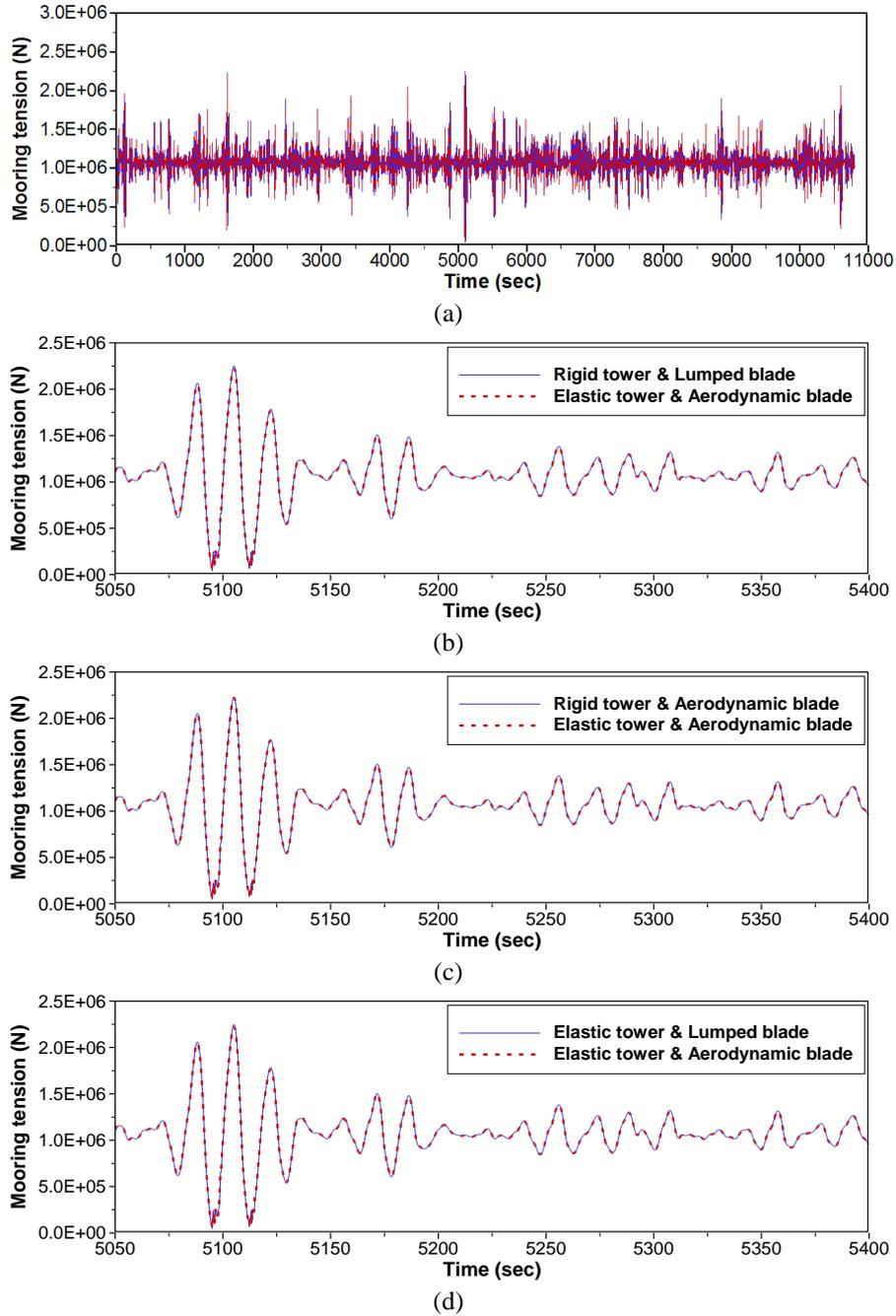
Fig. 11 (a) Comparison of mooring line tension in sea state 8 (full range), (b) Comparison of mooring line tension in sea state 8 (zoom range : case 1 vs 4), (c) Comparison of mooring line tension in sea state 8 (zoom range : case 2 vs 4) and (d) Comparison of mooring line tension in sea state 8 (zoom range : case 3 vs 4)
