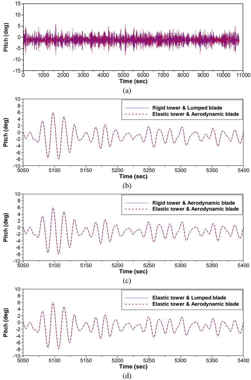
Fig. 10 (a) Comparison of pitch in sea state 8 (full range), (b) Comparison of pitch in sea state 8 (zoom range : case 1 vs 4), (c) Comparison of pitch in sea state 8 (zoom range : case 2 vs 4) and (d) Comparison of pitch in sea state 8 (zoom range : case 3 vs 4)
