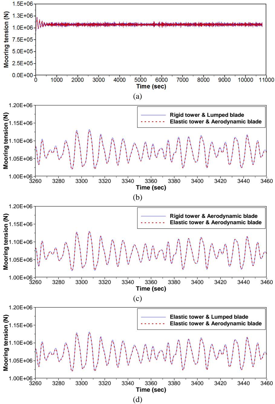
Fig. 6 (a) Comparison of mooring line tension in sea state 5 (full range), (b) Comparison of mooring line tension in sea state 5 (zoom range : case 1 vs 4), (c) Comparison of mooring line tension in sea state 5 (zoom range : case 2 vs 4) and (d) Comparison of mooring line tension in sea state 5 (zoom range : case 3 vs 4)
