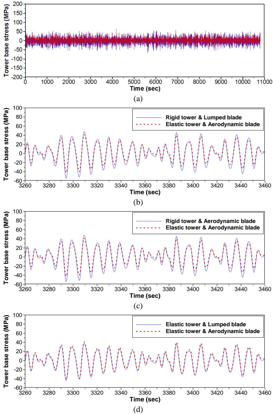
Fig. 7 (a) Comparison of tower base stress in sea state 5 (full range), (b) Comparison of tower base stress in sea state 5 (zoom range : case 1 vs 4), (c) Comparison of tower base stress in sea state 5 (zoom range : case 2 vs 4) and (d) Comparison of tower base stress in sea state 5 (zoom range : case 3 vs 4)
