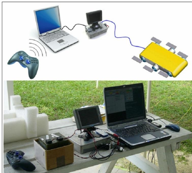
Fig. 11 General experimental setup with Aqua
