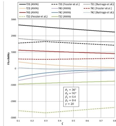
Fig. 24 Effects of  $\gamma$  on non-diagonal terms of the LJF matrix for a Y-T joint
