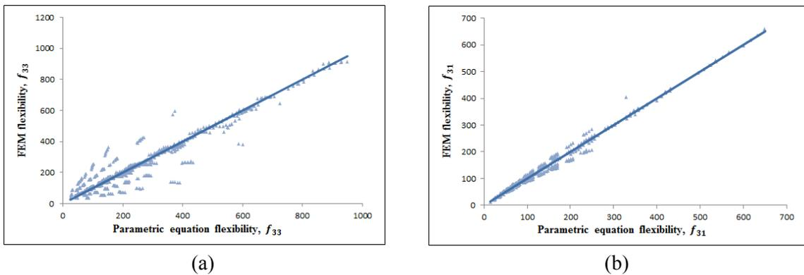
Fig. 5 (a) Comparison of parametric equation with the FE results for  $f_{33}$  and (b) Comparison of parametric equation with the FE results for  $f_{31}$
