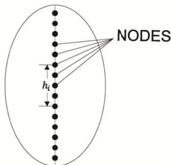
Fig. 2 Locations of the nodes on the intersection areas between the chord and the braces used to calculate the rotations
