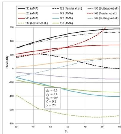
Fig. 22 Effects of  $\theta_1$  on non-diagonal terms of the LJF matrix for a Y-T joint
