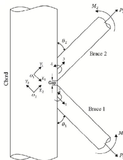
Fig. 1 Definition of local coordinate systems and positive directions for degrees of freedom
