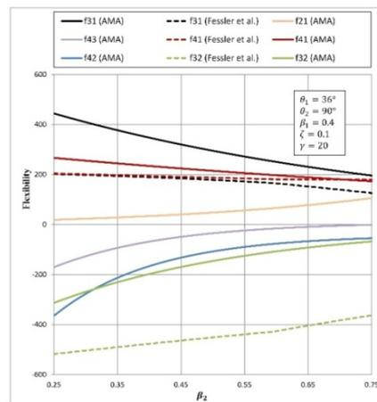
Fig. 21 Effects of  $\beta_2$  on non-diagonal terms of the LJF matrix for a Y-T joint
