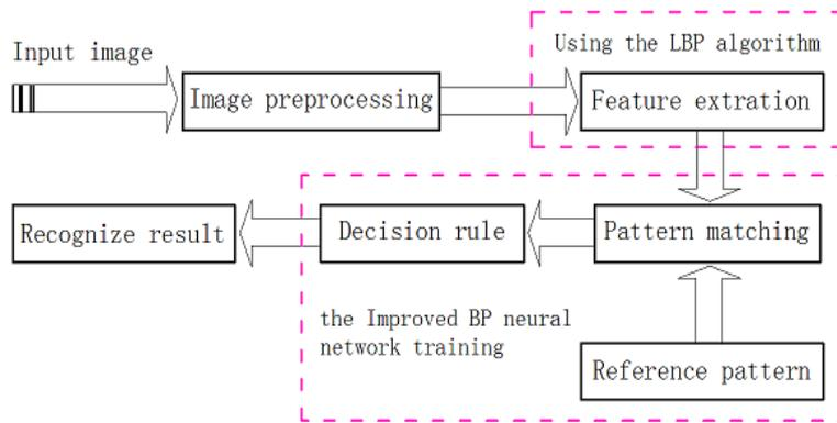
Fig. 7 The flowchart of ship wake image classification
