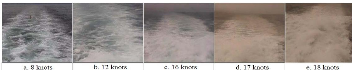
Fig. 4 Ship wake patterns at different speeds
