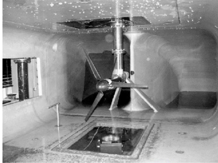
Fig. 2 The model tidal turbine in the cavitation tunnel experiment, taken from Bahaj *et al.* (2007)
