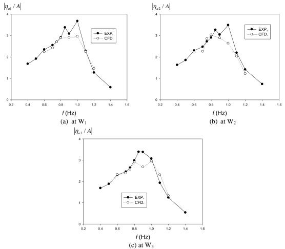
Fig. 6 Comparison of amplification factor between OpenFOAM numerical solutions and experimental results at different locations ( $W_1, W_2, W_3$ ) in the resonator for *R*=18.8 cm, 2*a*=10 cm and 2*b*=1 cm
