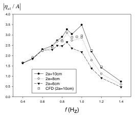
Fig. 11 Experimental results of amplification factor at the  $W_1$  position as a function of the gap width of the entrance for R=18.8 cm and 2b=1 cm
