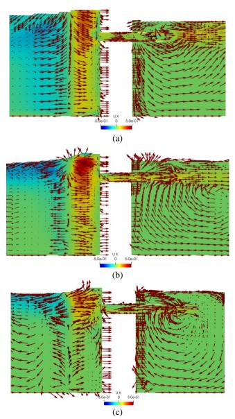
Fig. 9 Flow visualization near the resonator and water channel for frequency 0.6Hz (a) 0.9Hz (b) 1.1Hz (c)
