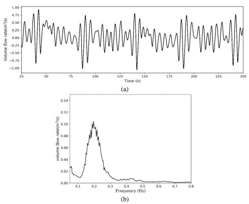
Fig. 15 Time history of volume flow rate (a) in the water channel and its amplitude spectra (b)
