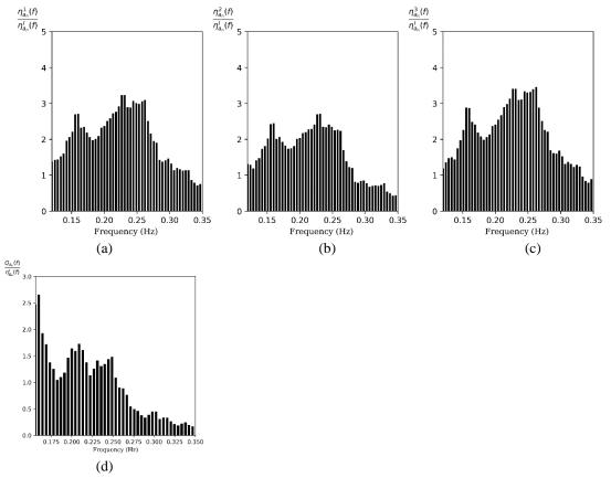
Fig. 16 Amplification factor of surface elevations in a resonator and volume flow rate through a water channel from irregular wave test
