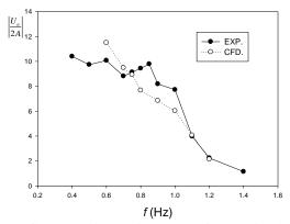
Fig. 8 Comparison of channel flow velocity against wave frequencies between OpenFOAM numerical solutions and experimental results for R=18.8 cm, 2a=10 cm, and 2b=1 cm
