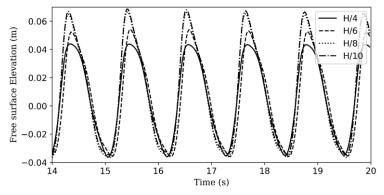
Fig. 3Time history of surface elevation at the position  $W_3$  in the resonator for different mesh refinements (f =0.9 Hz)
