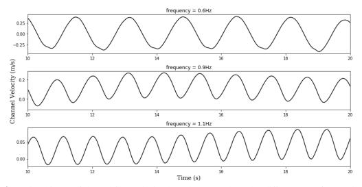
Fig. 7 Time history of channel flow velocity through a water channel at different wave frequencies
