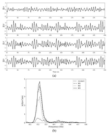
Fig. 14 Time history of both the incident wave and surface elevations in a resonator (a), and its wave spectra (b)
