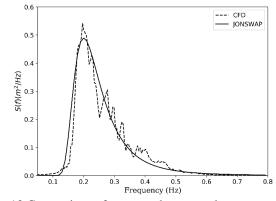
Fig. 13 Comparison of target and generated wave spectrum
