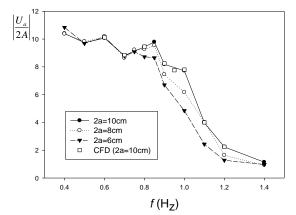
Fig. 12 Experimental results of flow velocity at the water channel as a function of the gap width of the entrance for R=18.8 cm and 2b=1 cm
