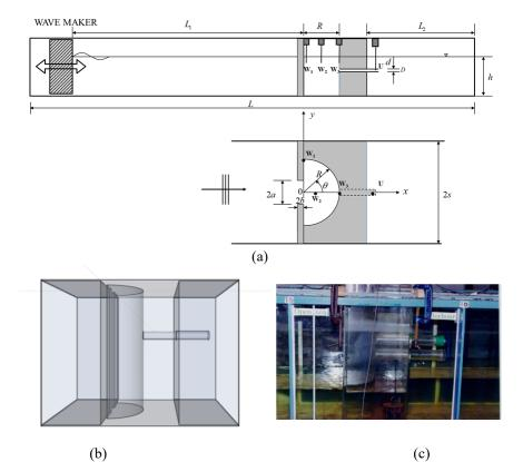
Fig. 2 Schematic view (a), 3D sketch (b), and photograph (c) of the experimental setup at a 2D wave tank
