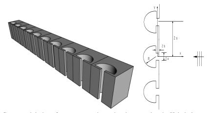
Fig. 1 Conceptual design of a seawater exchange breakwater using the Helmholtz resonator
