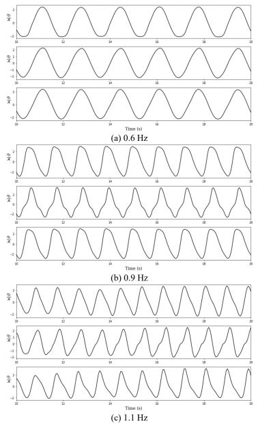
Fig. 5 Time history of free-surface elevation at three different positions ( $W_1$ , $W_2$ , $W_3$ ) for different wave frequencies f = 0.6, 0.9, 1.1 Hz
