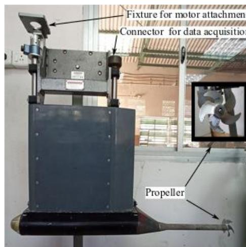
Fig. 15 Experimental setup to test open water characteristics of propeller
