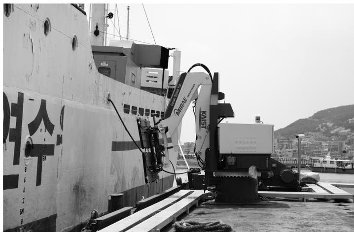
Fig. 7 Sea trial of the automatic ship-to-ship mooring system
