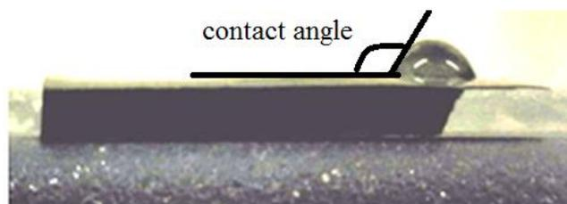
Fig. 3 Contact angle test image
