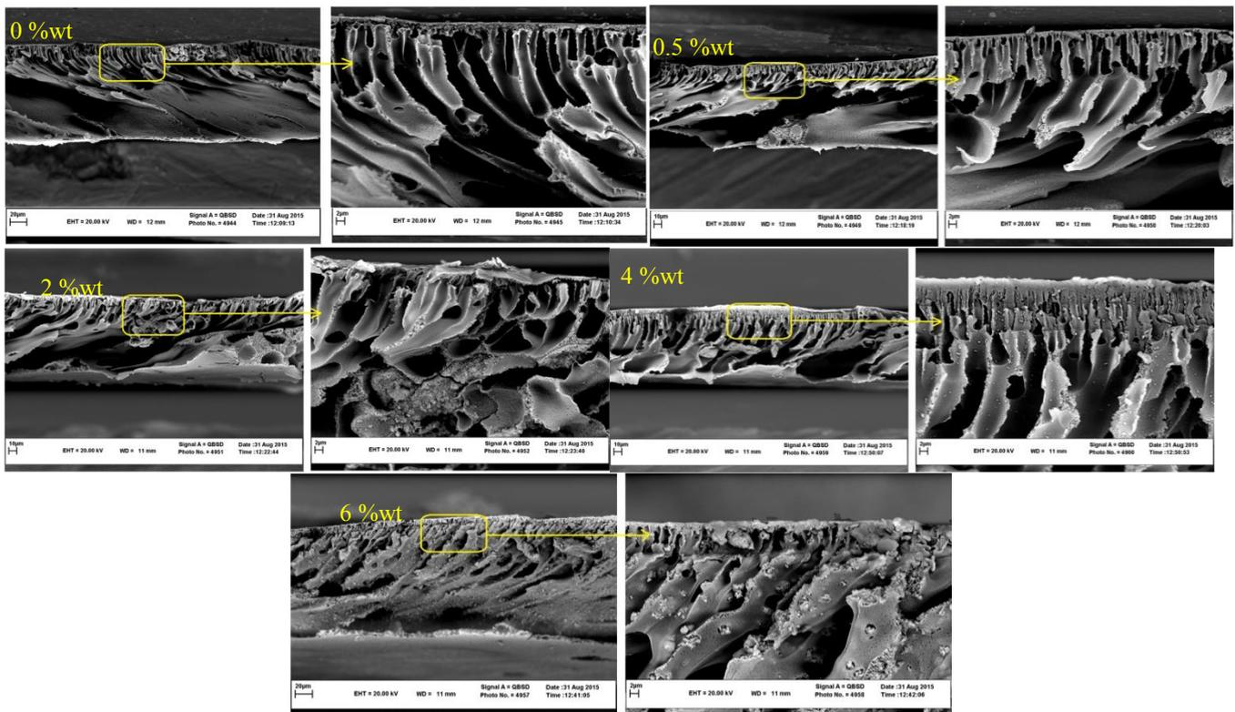
Fig. 4 SEM images of the cross-sectional morphologies of the nanocomposite membrane polyethersulfone / titanium / copper dioxide with different percentages of nanoparticles
