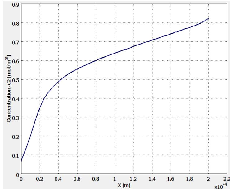
Fig. 4 Concentration profile of water vapor in the gas phase
