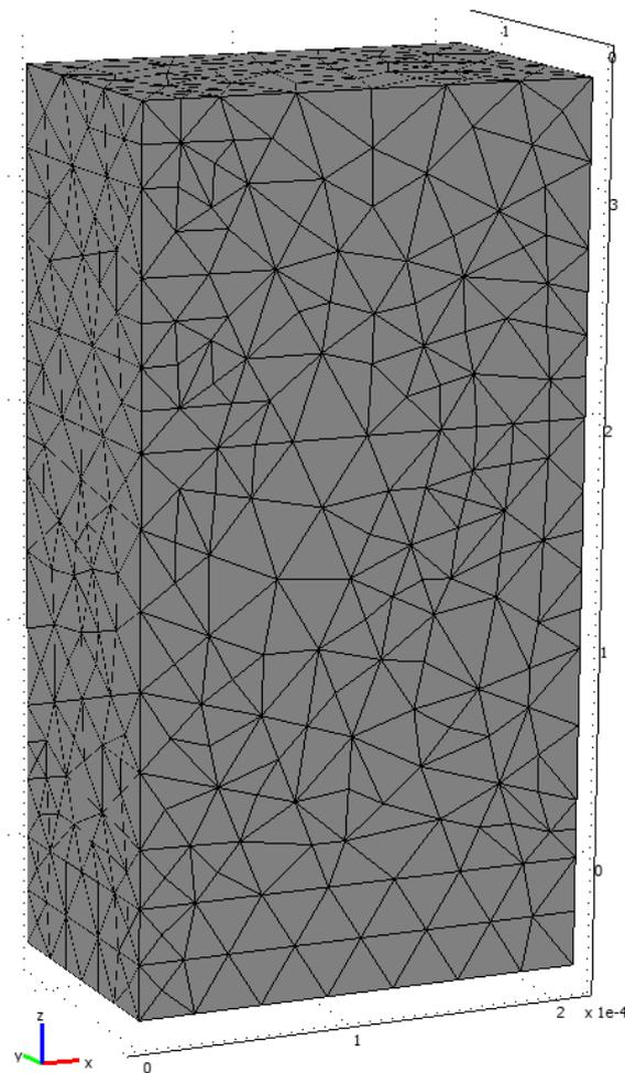
Fig. 3 Meshed geometry used in numerical simulations
