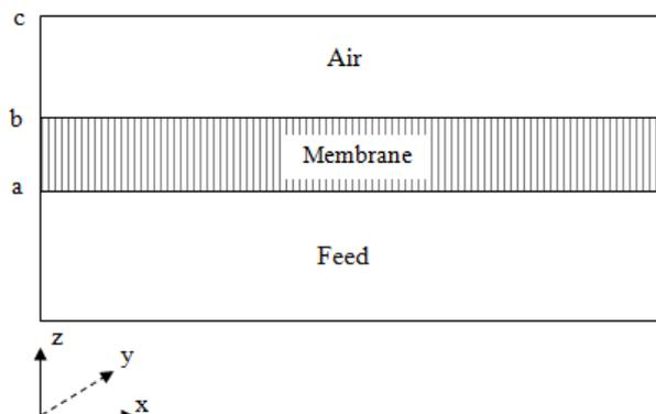
Fig. 1 Three subdomains considered in simulation of membrane evaporation process
