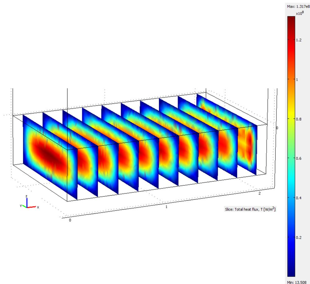
Fig. 7 Distribution of total heat flux in the feed phase
