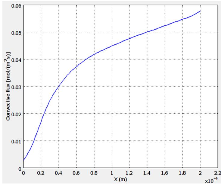
Fig. 5 Profile of convective mass transfer flux in the gas phase
