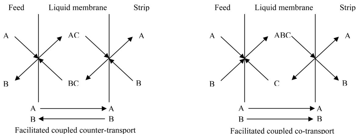
Fig. 1 Facilitated coupled transport of ionic solutes through a liquid membrane
