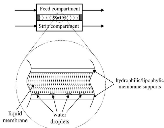
Fig. 4 Schematization of the permeation module and zoom on the SSwLM evidencing LM phase stratification on water droplets
