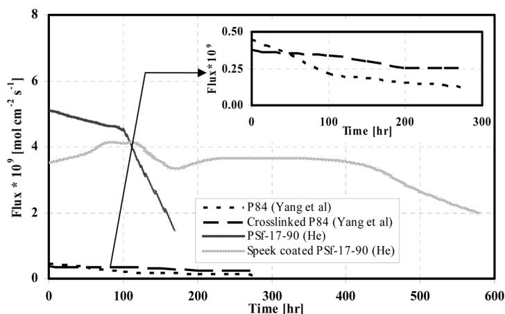
Fig. 2 Fluxes vs. time of SLMs assembled with original and modified membrane supports (elaborated from Yang *et al.* (2007) and He (2008))
