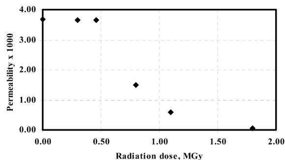
Fig. 5 Permeability vs radiation dose for Am(III) transport across the SLM used (from Ansari et al. (2007))
