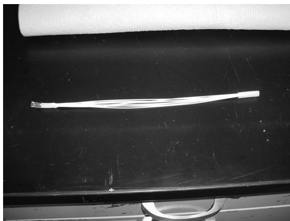
Photo 1 Fabricated hollow fiber membrane module with open side on the right and dead end on the left
