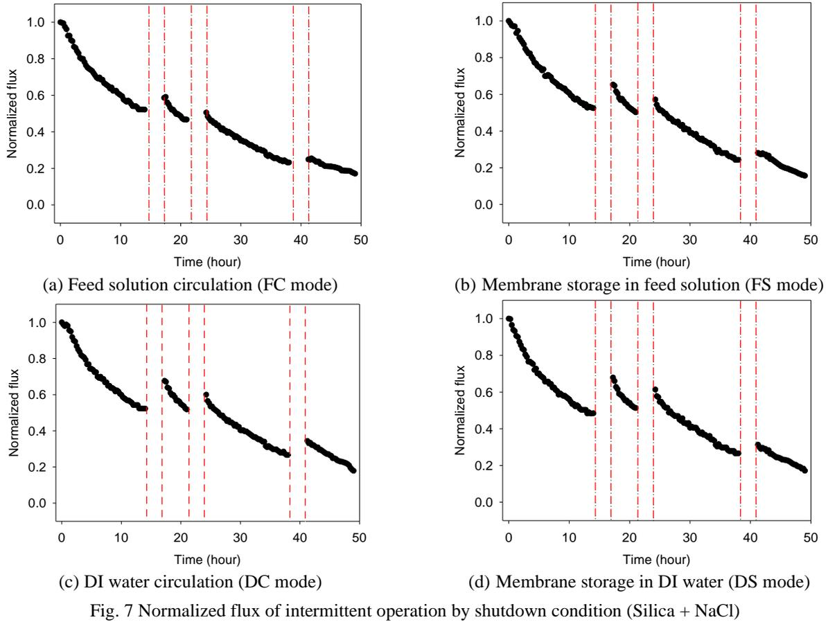
Fig. 7 Normalized flux of intermittent operation by shutdown condition (Silica + NaCl)
