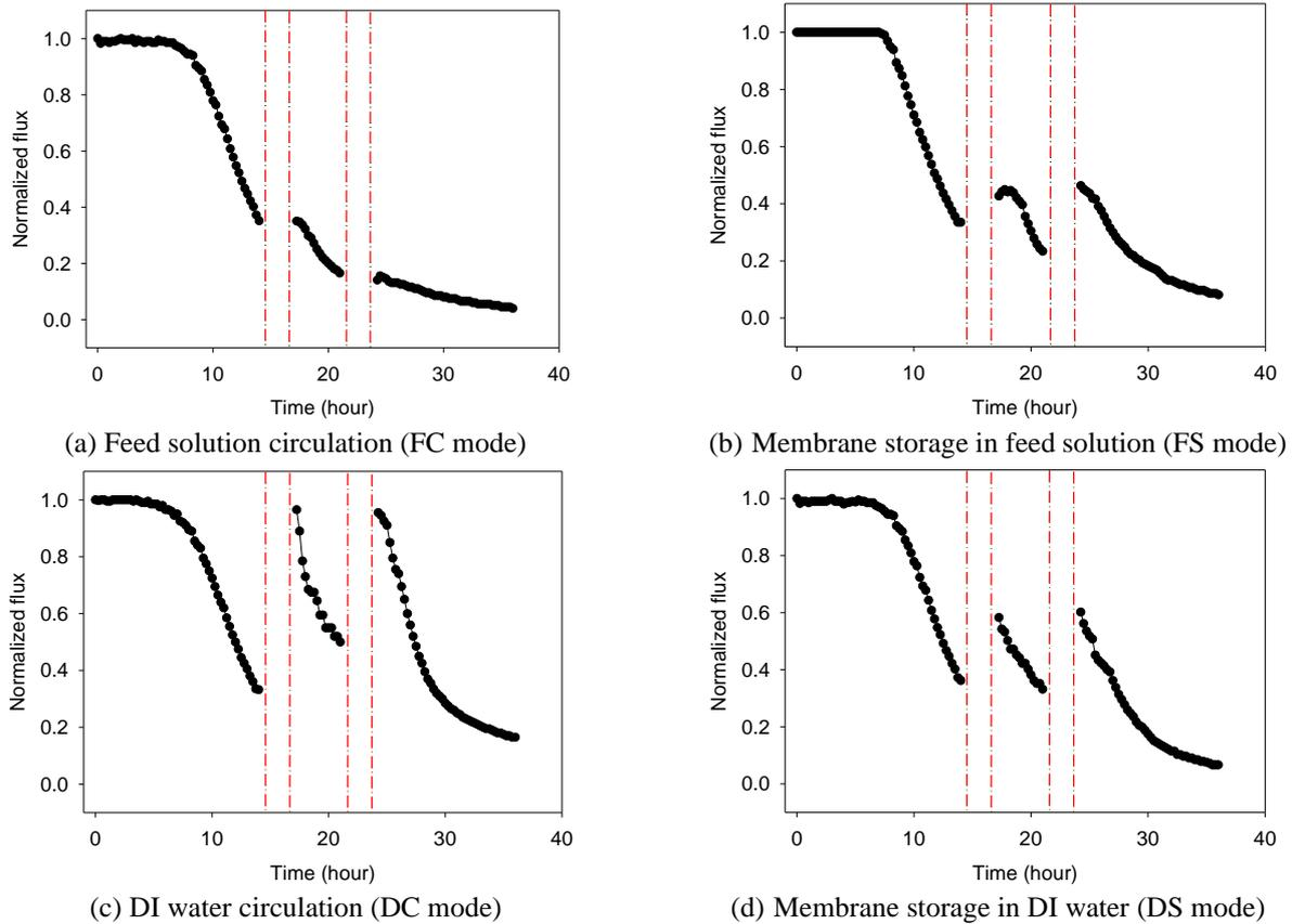
Fig. 4 Normalized flux of intermittent operation by shutdown condition ( $\text{CaSO}_4$ )
