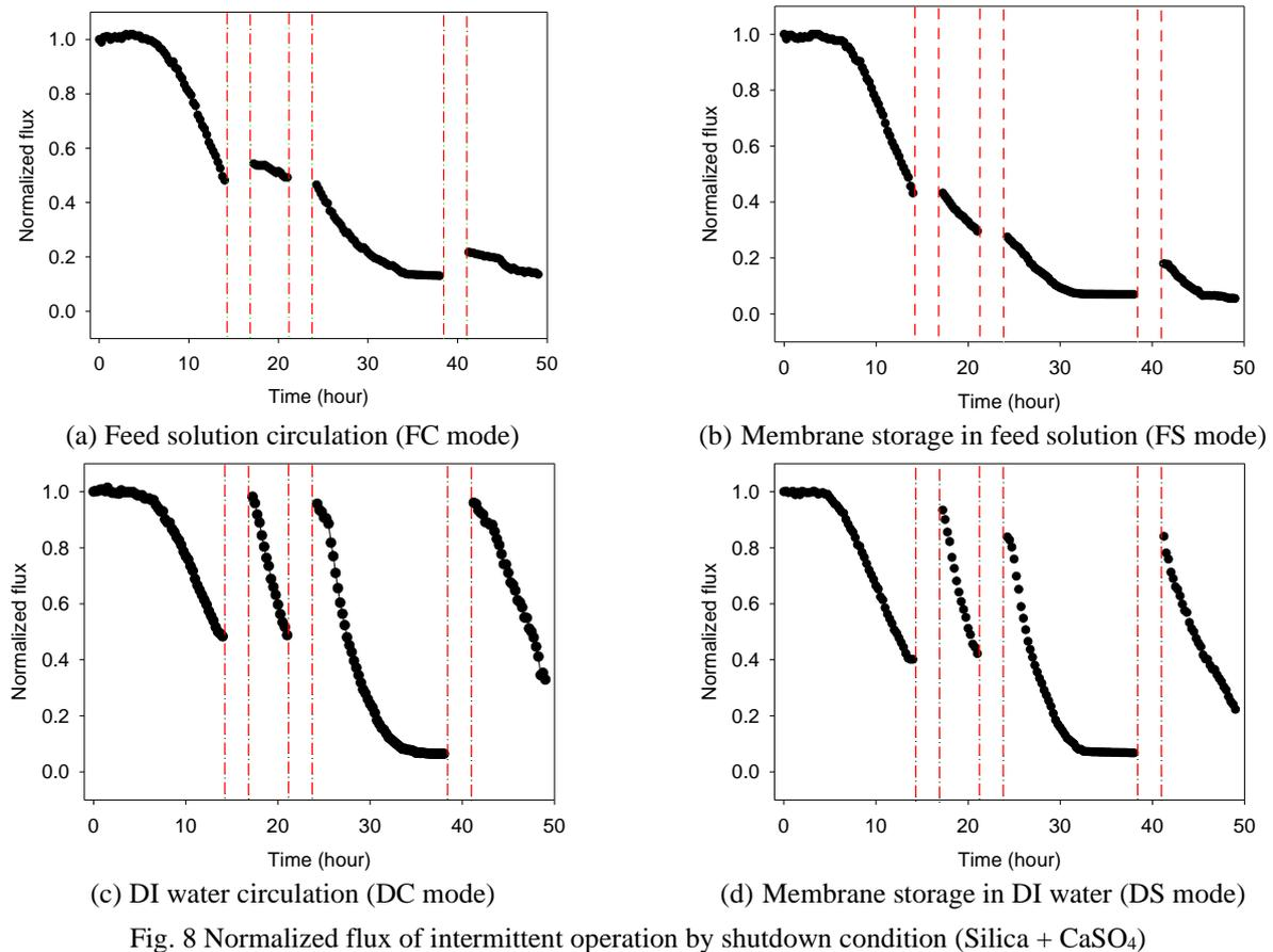
Fig. 8 Normalized flux of intermittent operation by shutdown condition (Silica + CaSO<sub>4</sub>)
