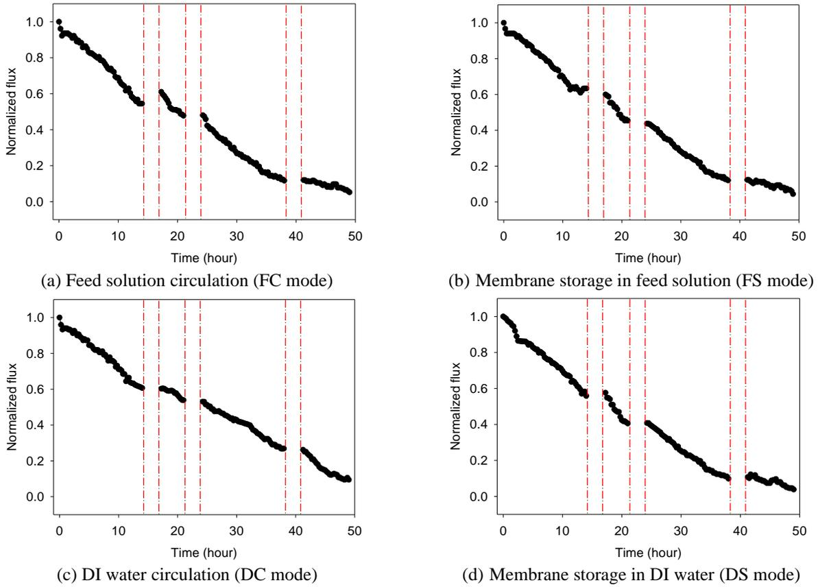
Fig.2 Normalized flux of intermittent operation by shutdown condition (NaCl + CaSO<sub>4</sub>)
