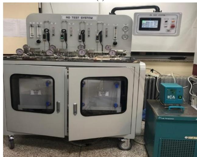
Fig. 1 Laboratory-scale intermittent RO experimental setup (a) schematic diagram (b) photography
