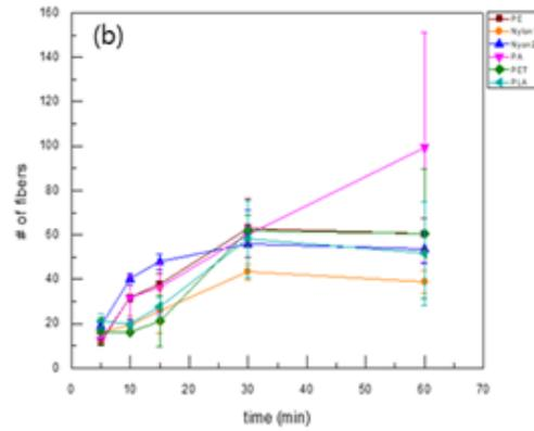
(b) The number of fibers released by different exposure time (5, 10, 15, 30 min, 1 hr)
