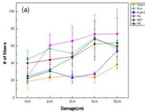
(a) The number of fibers released based on the size of damage (1, 2, 3, 5, 10 cm)
