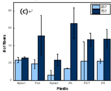
(c) The number of fibers released under various temperatures (25°C, 75°C)
