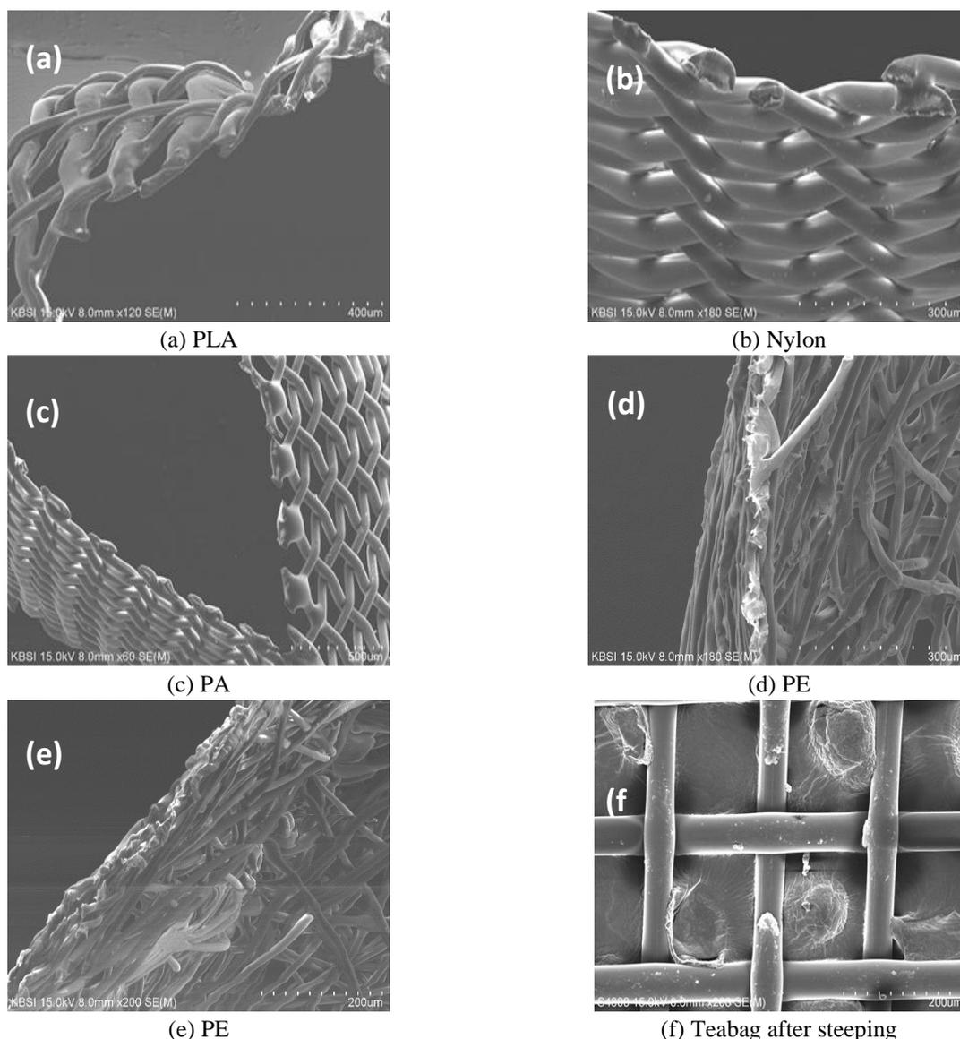
Fig. 1 SEM image of the cross section of damaged tea bags of various chemical compositions
