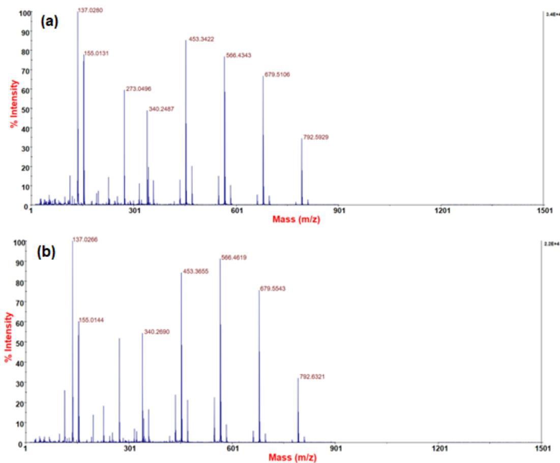
Fig. 6 MALDI-MS analysis of filtered samples from teabags composed of nylon (Nylon 1 and Nylon 2)
