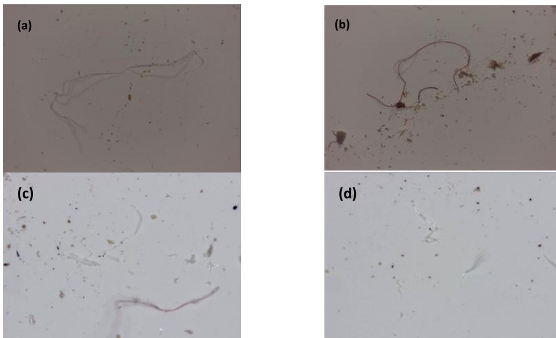
Fig. 2 Optical image of micro plastic fiber and particle release from the damaged teabags. The different color particles and fibers show the released fibers from the damaged teabags
