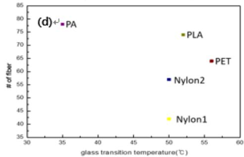
(d) Correlation between the glass transition temperature and fiber release
