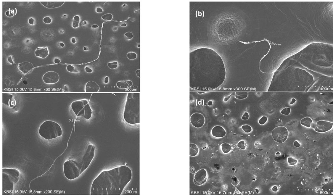
Fig. 5 SEM imaging of filtered water for the tea bags; The numbers in (a), (b), and (c) show the thickness of the released fibrous microplastics
