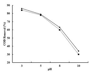
Fig. 3 Effect of different pH on COD removal efficiency in Fenton method (PGU restaurant ( $\blacksquare$ ): Fe<sup>2+</sup>=1000 mg/L, H<sub>2</sub>O<sub>2</sub>=1000 mg/L; Shif Island ( $\blacklozenge$ ): Fe<sup>2+</sup>=500 mg/L and H<sub>2</sub>O<sub>2</sub>=500 mg/L; Time=90 min)
