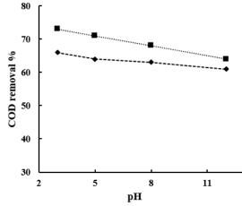
Fig. 7 Effect of different pH on COD removal efficiency in UV/TiO2 process (PGU restaurant ( $\blacklozenge$ ): TiO<sub>2</sub> = 1 g/L and Shif Island ( $\blacksquare$ ): TiO<sub>2</sub> = 1 g/L; Time=180 min).
