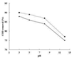
Fig. 5 Effect of different pH on COD removal efficiency in UV/H<sub>2</sub>O<sub>2</sub> process (PGU restaurant ( $\blacklozenge$ ): H<sub>2</sub>O<sub>2</sub> = 1500 mg/L and Shif Island ( $\blacksquare$ ): H<sub>2</sub>O<sub>2</sub> = 750 mg/L; Time = 180 min).
