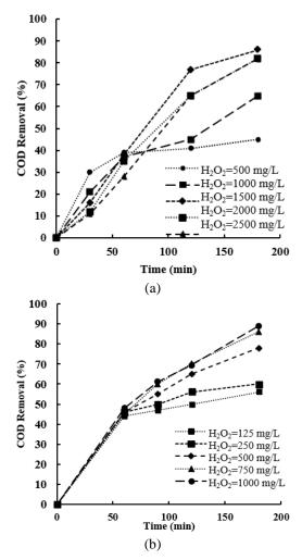
Fig. 4 Effect of time and various  $H_2O_2$  concentrations on COD removal efficiency of: (a) PGU restaurant and (b) Shif Island grey water by UV/H<sub>2</sub>O<sub>2</sub> process; at initial pH = 8
