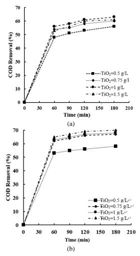
Fig. 6 Effect of time and various  $TiO_2$  concentrations on COD removal efficiency of: (a) PGU restaurant and (b) Shif Island grey water by UV/  $TiO_2$  process; at initial pH
