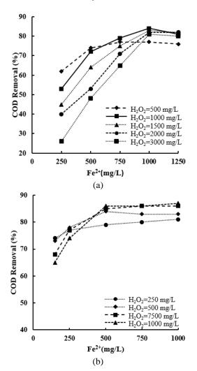
Fig. 2 Effect of various  $H_2O_2$  and  $Fe^{2+}$  concentration on COD removal efficiency of: (a) PGU restaurant and (b) Shif Island grey water at pH= 3 & Time=90 min
