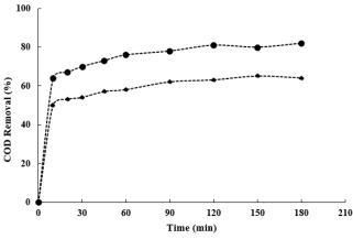
Fig. 1 Effect of time in Fenton process for COD removal of grey waters of Shif Island ( $\bullet$ ) and PGU restaurant ( $\bullet$ ) (pH = 3, Fe2+ = 250 mg/L and H<sub>2</sub>O<sub>2</sub> = 500 mg/L)
