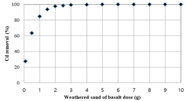
Fig. 4 Effect of weathered sand of basalt dosage on Cd adsorption capacity
