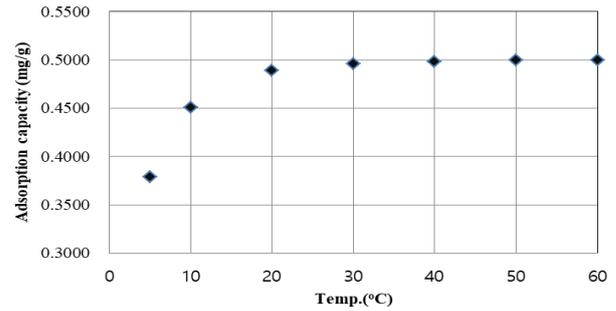
Fig. 6 Effect of adsorption temperature on Cd adsorption capacity
