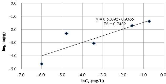
Fig. 12 The Freundlich sorption isotherm (pH 8, WSB dose 2 g, adsorption time 180 min, WSB particle size 251~355  $\mu\text{m}$  and temperature 30°C)
