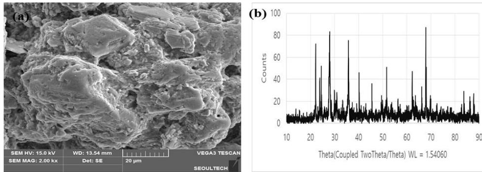
Fig. 1 Scanning electron micrograph (a) and X-ray diffraction (b) of the WSB
