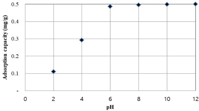
Fig. 3 Effect of pH on Cd adsorption capacity
