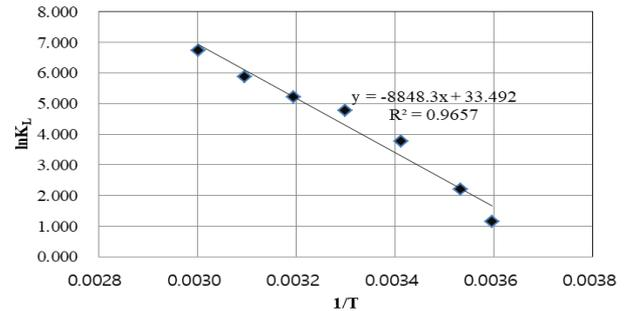
Fig. 7 Van't Hoff plot for the Cd adsorption onto WBS
