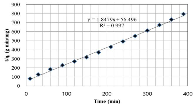
Fig. 10 Pseudo-second-order kinetic plot for the adsorption of Cd onto WSB (pH 8, initial Cd concentration 1.0 mg/L, WSB dose 2 g, adsorption time 180 min, WSB particle size 251~355  $\mu\text{m}$  and temperature 30°C)
