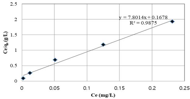
Fig. 11 The Langmuir sorption isotherm (pH 8, WSB dose 2 g, adsorption time 180 min, WSB particle size 251~355  $\mu\text{m}$  and temperature 30°C)
