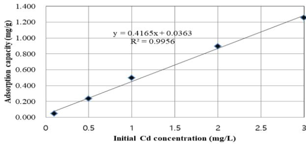
Fig. 8 Effect of initial Cd concentration on Cd adsorption capacity
