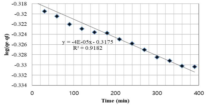
Fig. 9 Pseudo-first-order kinetic plot for the adsorption of Cd onto WSB (pH 8, initial Cd concentration 1.0 mg/L, WSB dose 2 g, adsorption time 180 min, WSB particle size 251~355  $\mu\text{m}$  and temperature 30°C)
