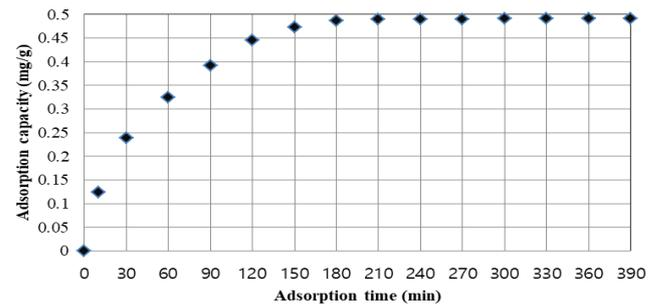
Fig. 2 Effect of contact time on Cd adsorption capacity
