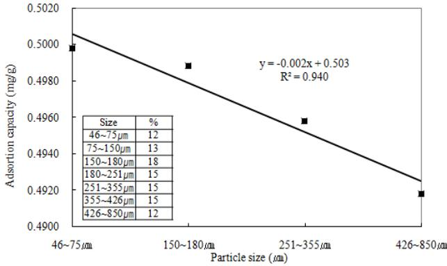
Fig. 5 Effect of weathered sand of basalt particle size on Cd adsorption capacity
