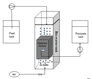
Fig. 1 Schematic representation of laboratory Submerged Membrane Bioreactor (SMBR)  $\bigcirc$  Influent pump,  $\bowtie$  Air flow meter,  $\bigcirc$  Effluent (permeate) pump
