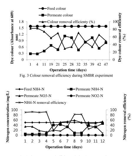
Fig. 4 Nitrogen removal efficiency during SMBR experiment
