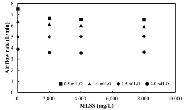
Fig. 3 Effects of MLSS concentration on the quantity of air flow rate according to hydraulic pressure
