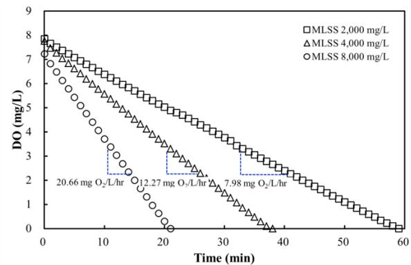
Fig. 4 Oxygen uptake rate according to MLSS concentration
