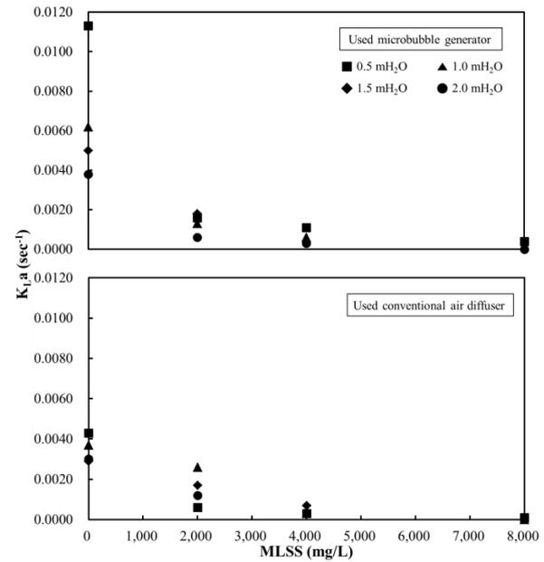
Fig. 6 Effects of MLSS concentration on  $K_{L,a}$  according to hydraulic pressure
