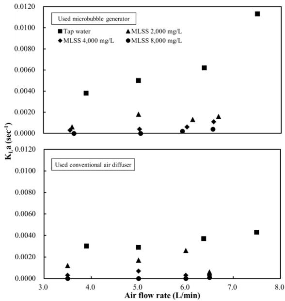
Fig. 5 Effects of the quantity of air flow rate on  $K_{L,a}$  according to MLSS concentration
