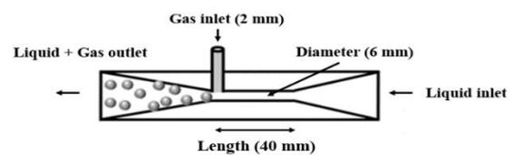
Fig. 2 Schematic diagram of ejector type venturi nozzle
