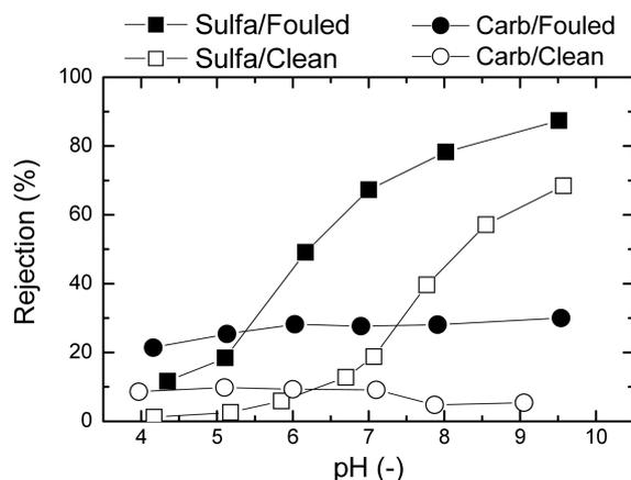
Fig. 6 Sulfamethoxazole and carbamazepine rejection by clean and fouled TFC-SR2 membranes as a function of pH. (Electrolyte solution contains: 20 mM NaCl, 1 mM NaHCO<sub>3</sub>, 1 mM CaCl<sub>2</sub>; crossflow velocity 30.4 cm/s; fouling was developed for 18 hrs with feed solution containing 20 mg/L humic acids.)
