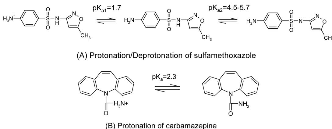
Fig. 2 Protonation/deprotonation of (A) sulfamethoxazole and (B) carbamazepine
