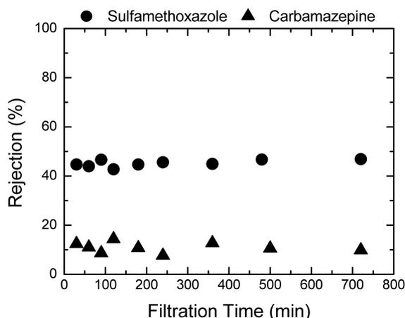
Fig. 3 Rejection of sulfamethoxazole, and carbamazepine by the TFC-SR2 membrane as a function of time (pH  $\approx$  8.0)
