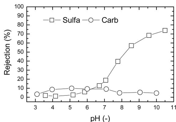
Fig. 4 Rejection of sulfamethoxazole and carbamazepine by the TFC-SR2 membrane as a function of solution pH
