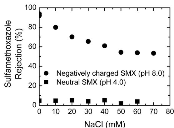
Fig. 5 Sulfamethoxazole rejection by the TFC-SR2 membrane as a function ionic strength at pH 8.0 and 4.0
