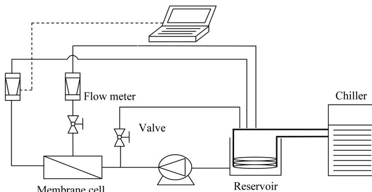
Fig. 1 Schematic diagram of the NF/RO filtration test unit
