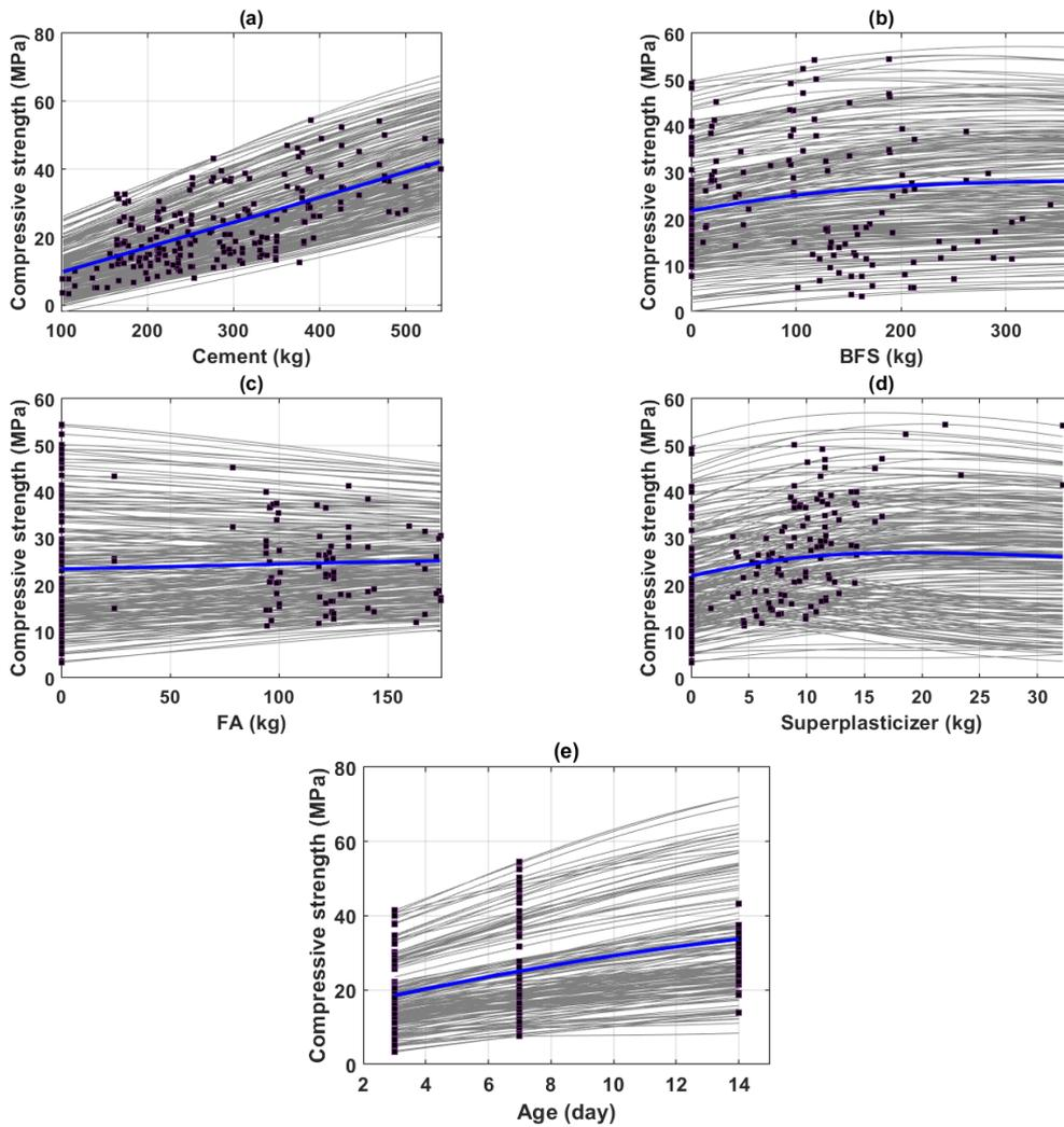
Fig. 5 Input variables exhibited a positive effect to the early compressive strength of HPC: (a) cement (b) blast furnace slag (c) fly ash (d) superplasticizer and (e) testing age
