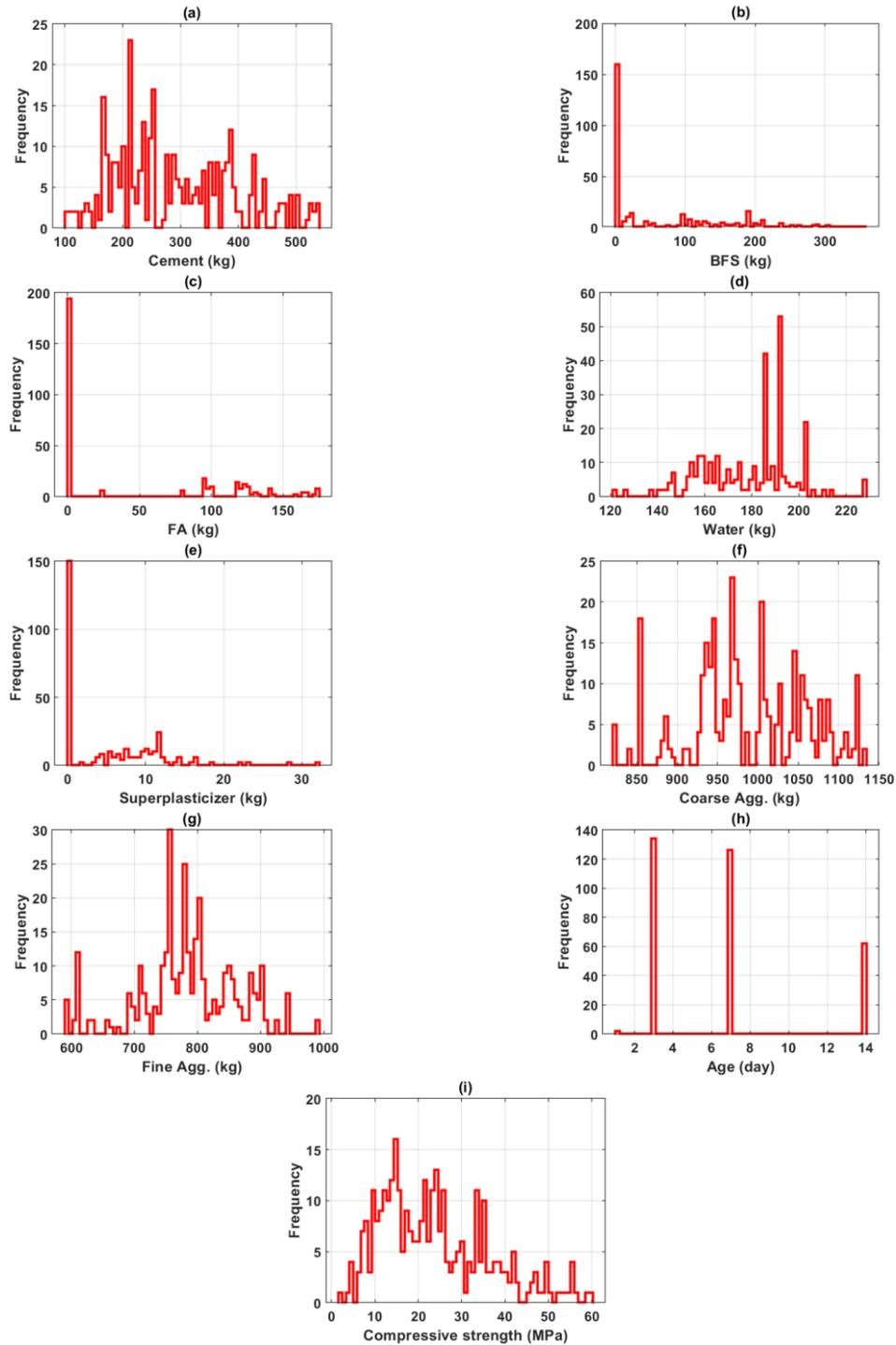
Fig. 1 Histogram including the ranges and frequencies of all the components in the database: (a) cement (b) blast furnace slag (c) fly ash (d) water (e) superplasticizer (f) coarse aggregate (g) fine aggregate (h) testing age (i) early compressive strength
