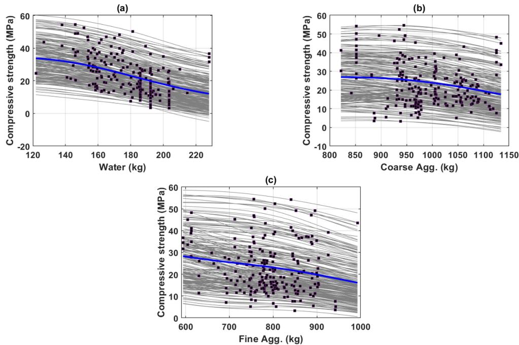
Fig. 6 Input variables exhibited a negative effect to the early compressive strength of HPC: (a) water; (b) coarse aggregate; and (c) fine aggregate
