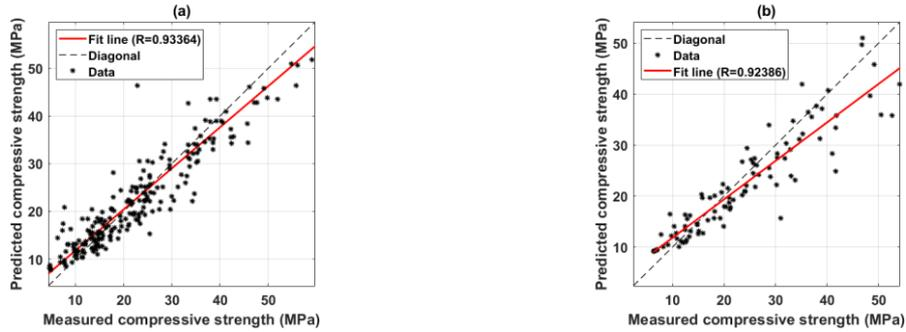
Fig. 4 Correlation graphs of SVR in predicting the early compressive strength of HPC: (a) training part and (b) testing part
