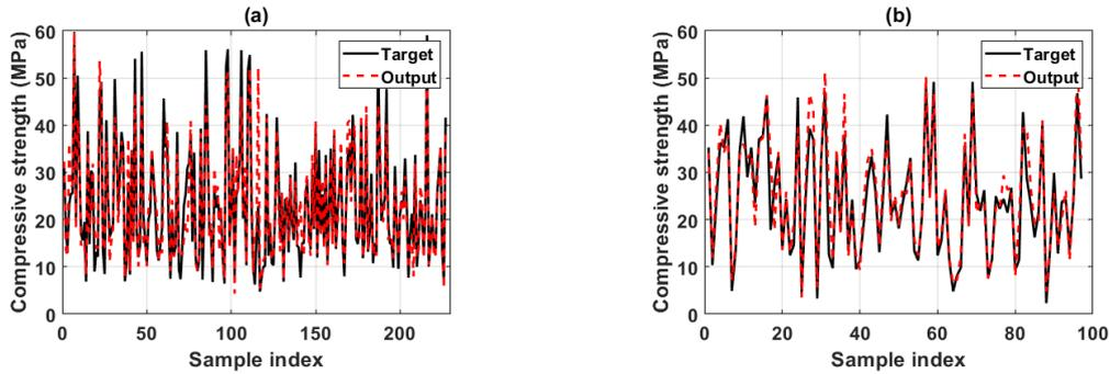
Fig. 2 Experimental and predicted values of early compressive strength of HPC with different datasets: (a) training part and (b) testing part
