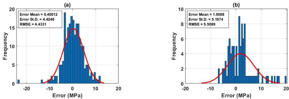
Fig. 3 Error histograms between experimental and predicted results of early compressive strength of HPC with different datasets: (a) training part and (b) testing part
