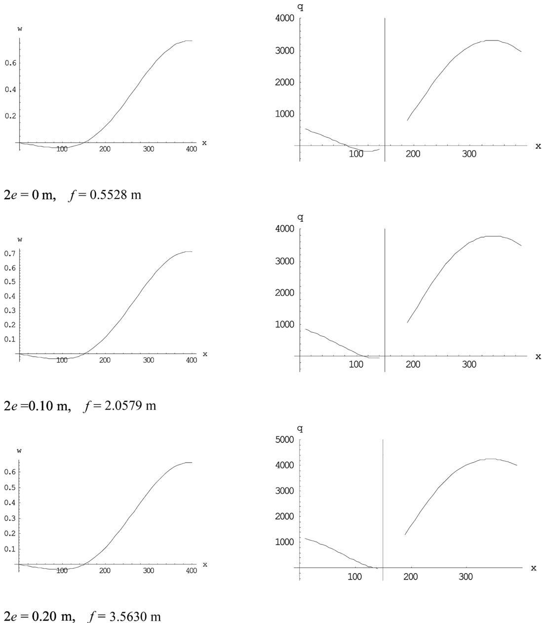
Fig. 16 Deck deformations and cables stresses for type-II bridge with slender pylons
