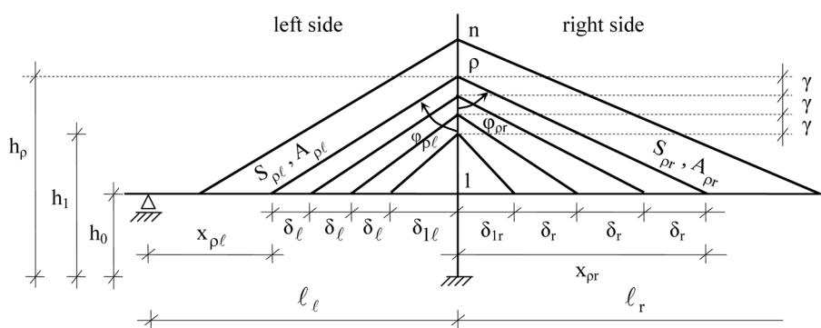
Fig. 6 Cable arrangement in a harp system
