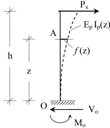
Fig. 3 Deformed configuration of the pylon
