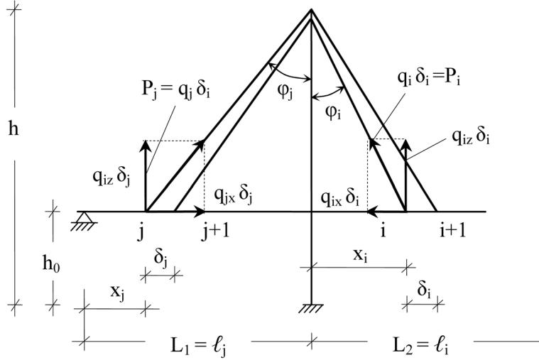
Fig. 5 Pylon force equilibrium due to a dense arrangement of cables
