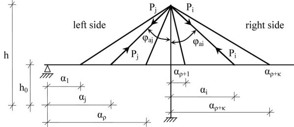
Fig. 4 Forces acting on the pylon due to the cables
