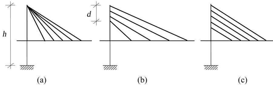
Fig. 1 Different systems of cables: (a) Fan, (b) Harp and (c) Parallel
