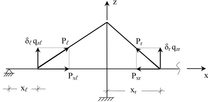
Fig. 9 Pylon stressing due to a dense arrangement of cables
