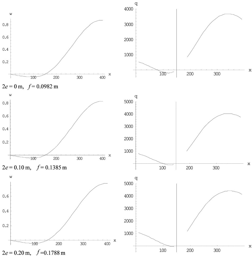
Fig. 11 Deck deformations and cables stresses for type-I bridge with stiff pylons
