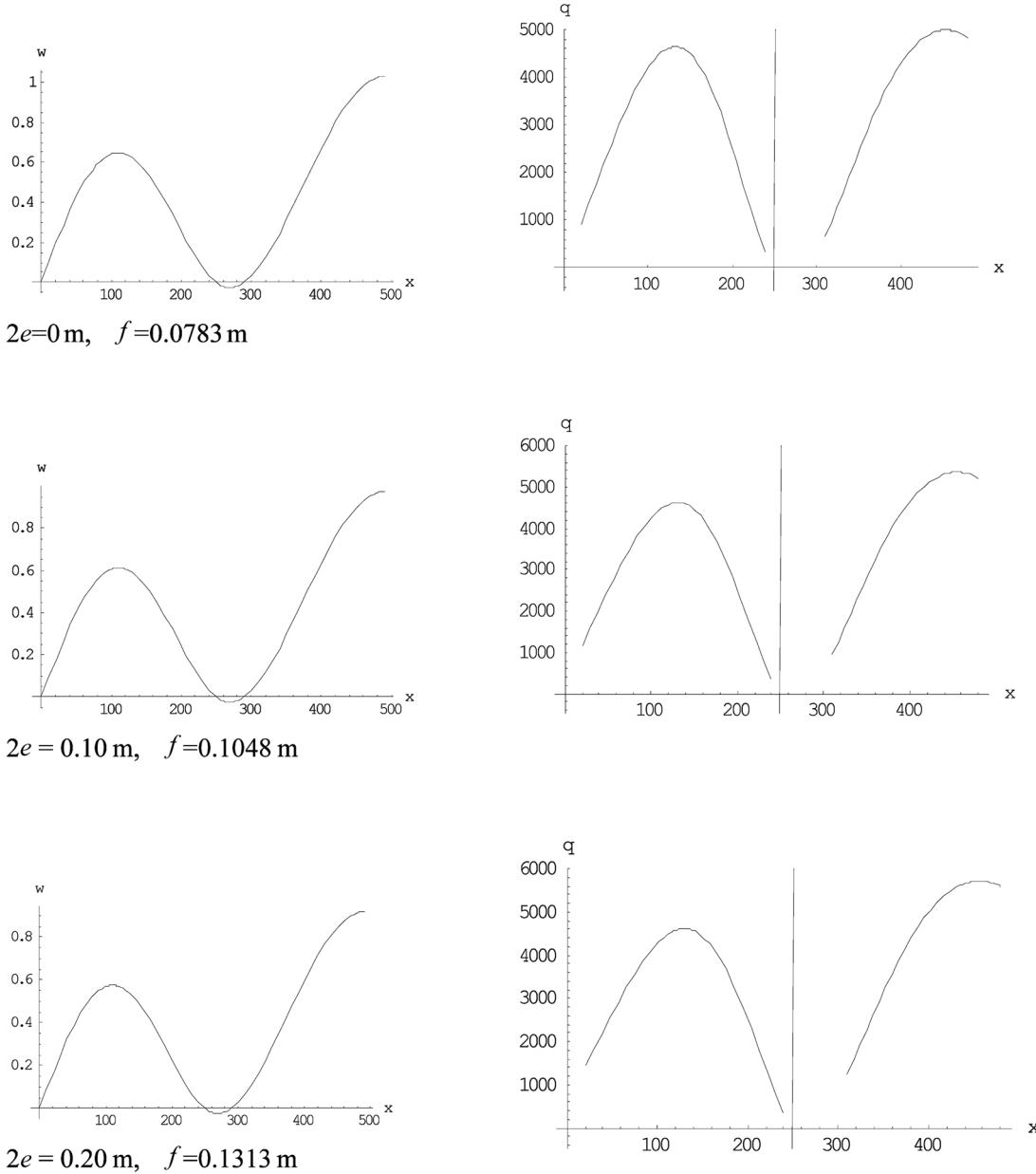
Fig. 13 Deck deformations and cables stresses for type-II bridge with stiff pylons
