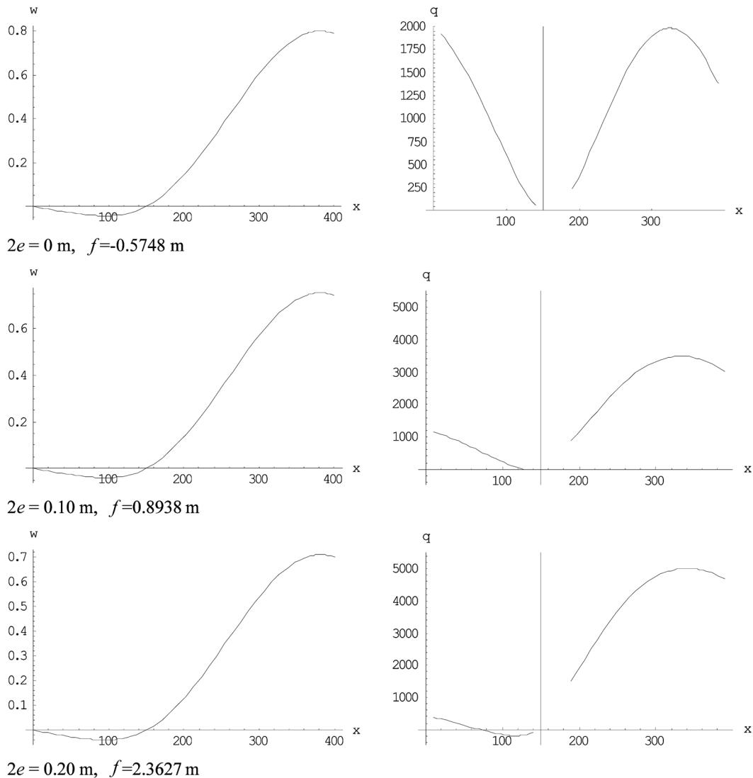
Fig. 10 Deck deformations and cables stresses for type-I bridge with slender pylons
