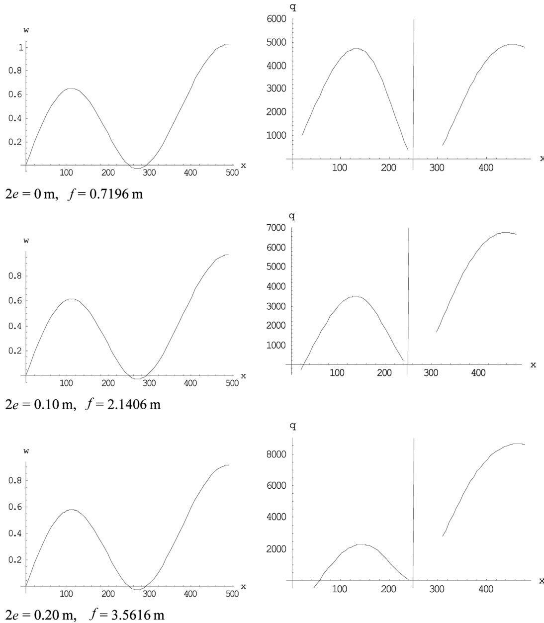
Fig. 12 Deck deformations and cables stresses for type-II bridge with slender pylons
