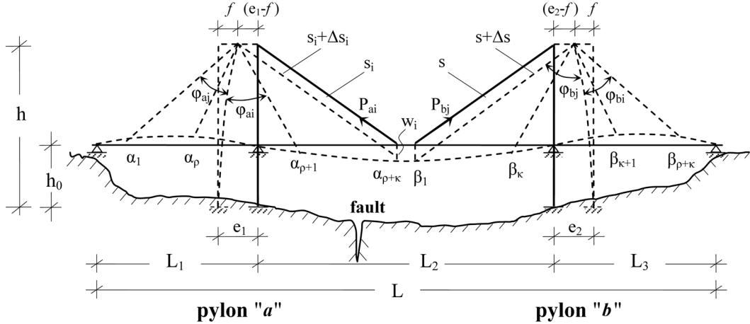
Fig. 2 Relative displacement of two neighboring pylons due to fault activation
