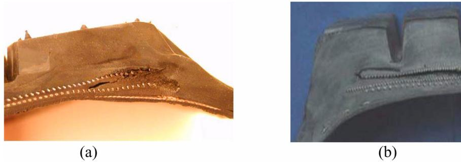
Fig. 1 Belt edge crack example from a steel belted radial tire: (a) a passenger car tire (Govindjee 2001), (b) a radial truck tire
