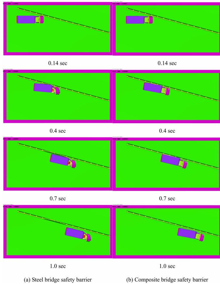
Fig. 7 Crash simulation of truck
