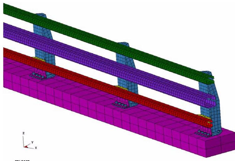
Fig. 2 Finite element modeling of bridge safety barrier
