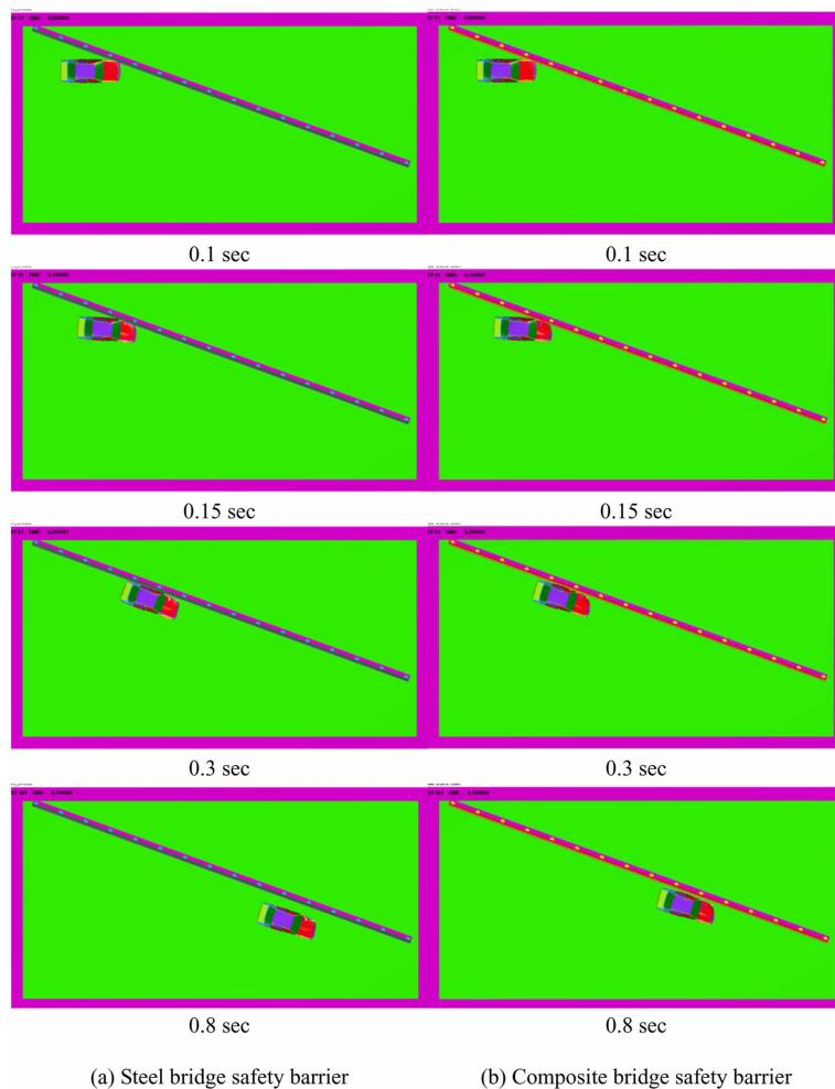
Fig. 6 Crash simulation of passenger car
