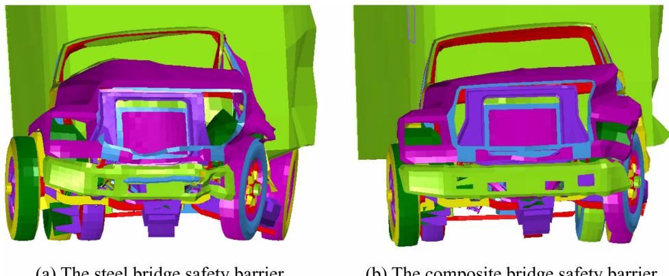
Fig. 4 Comparison of deformation shape of the truck
