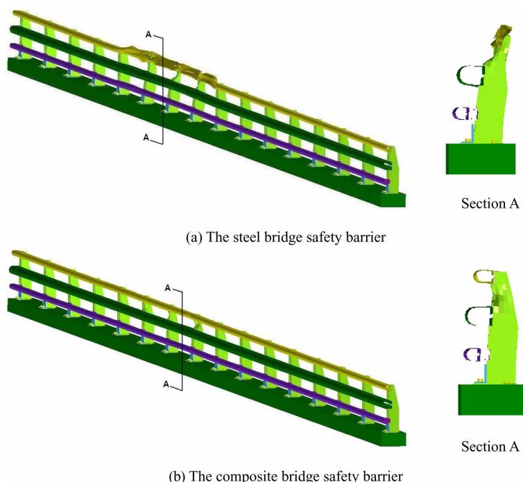
Fig. 5 Comparison of deformation shape of bridge safety barrier
