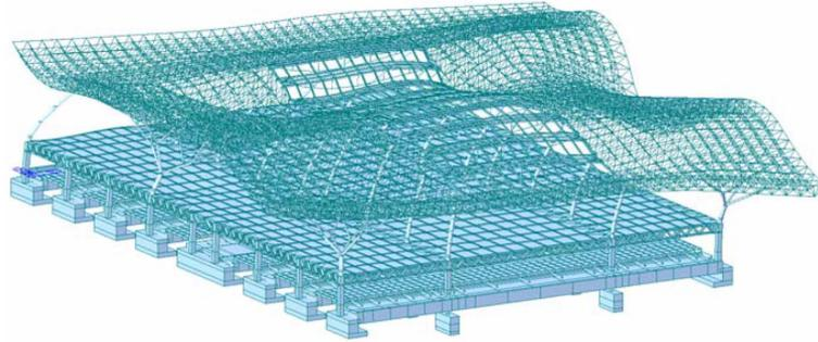
Fig. 6 The first mode shape of station (local vibration of roof,  $f=1.009$  Hz)
