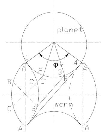
Fig. 3 Space phase relation of the coils on the worm
