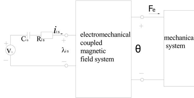
Fig. 2 Dynamic model of an electromechanical integrated toroidal drive
