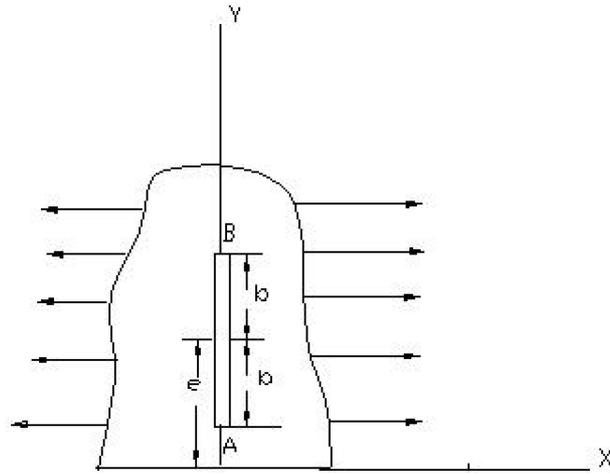
Fig. 1 Crack in semi-infinite plate
