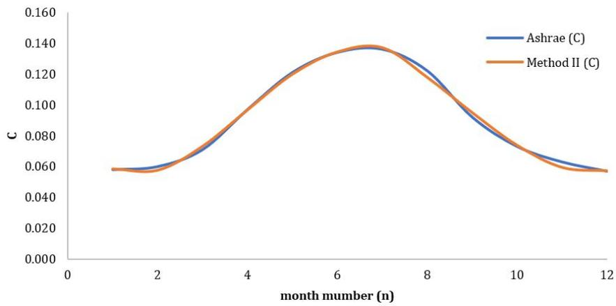
Fig. 7 Comparison of Ashrae constant C with Model II
