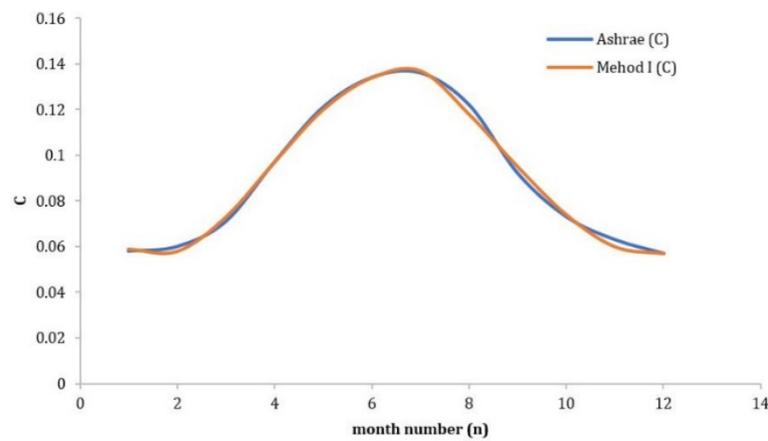
Fig. 4 Comparison of Ashrae constant C with Model I
