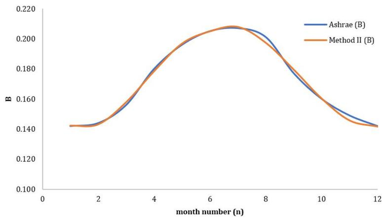
Fig. 6 Comparison of Ashrae constant B with Model II
