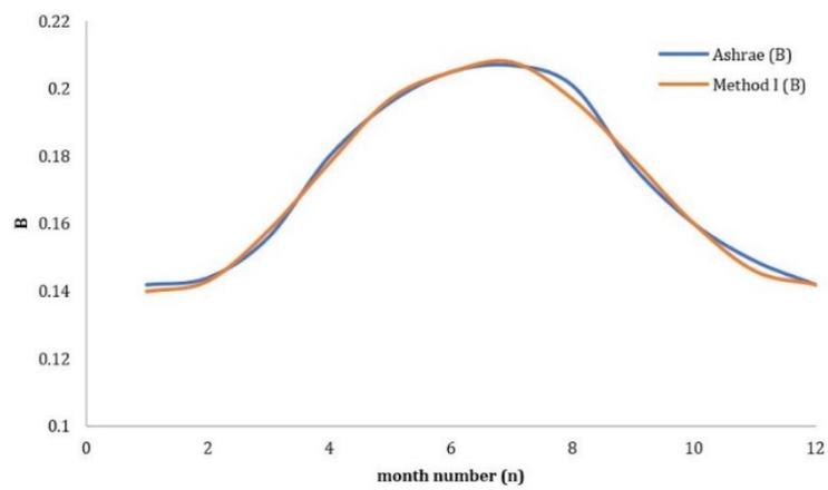
Fig. 3 Comparison of Ashrae constant B with Model I
