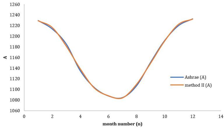
Fig. 5 Comparison of Ashrae constant A with Model II
