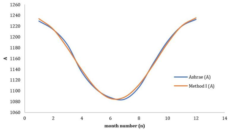
Fig. 2 Comparison of Ashrae constant A with Model I
